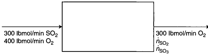
Figure 5.2 Flow diagram for Illustrative Example 5.7.
