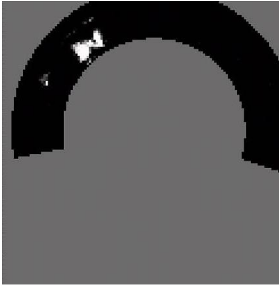
Fig. 7. Dead zones and pixel activity metric. The solid gray areas are a priori declared uninteresting. The bright white region is high pixel activity
