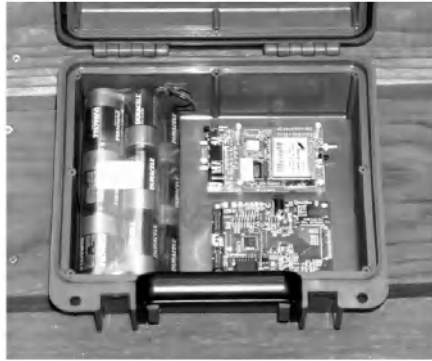
Fig. 8. View of interior of data logger being developed by Douglas Alden. Battery pack (to the left) provides power for data storage and transmission (electronics on right)
