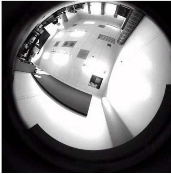
Fig. 4. Example of a panoramic image, taken using a zenith-looking fisheye lens
