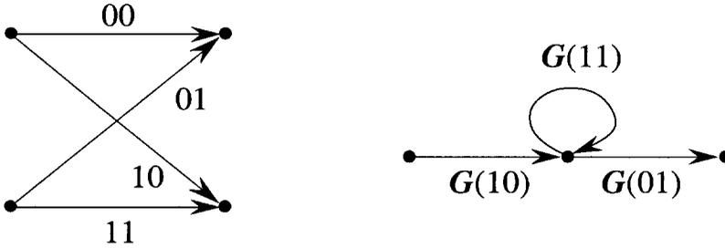
Figure 7.20: Trellis diagram of a TCM scheme with two states and  $m = 1$  (the branch labels are the components of  $\mathbf{c}$ ) and error state diagram.
