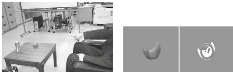
Fig. 11.8 Experimental example 2. When the user said, “Get that,” while pointing toward the object, the robot recognized the object in the rightmost figure as the one indicated by ‘that’ because it was being pointed at.
