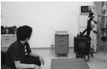
Fig. 11.7 Experimental example 1. When the user said, “Get that,” the robot recognized the object in the right figure as the one referenced by ‘that’ because it was close to the robot and in the direction of the user’s face.
