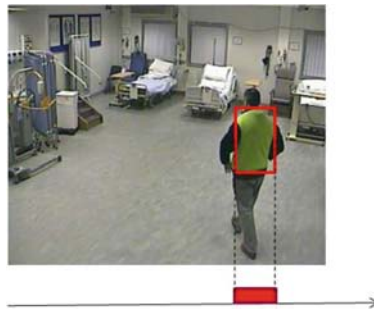
Fig. 7.3 The bounding box of a blob representing a person or part of a person is collapsed onto the horizontal axis. It will contribute to the profile of the scene for that specific category of people.
