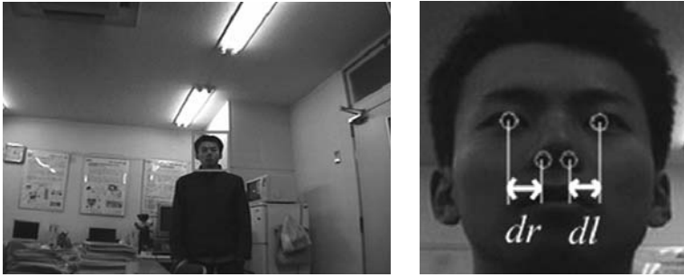
Fig. 11.14 Face image processing. Left: Face candidate. Right: Face direction computation.
