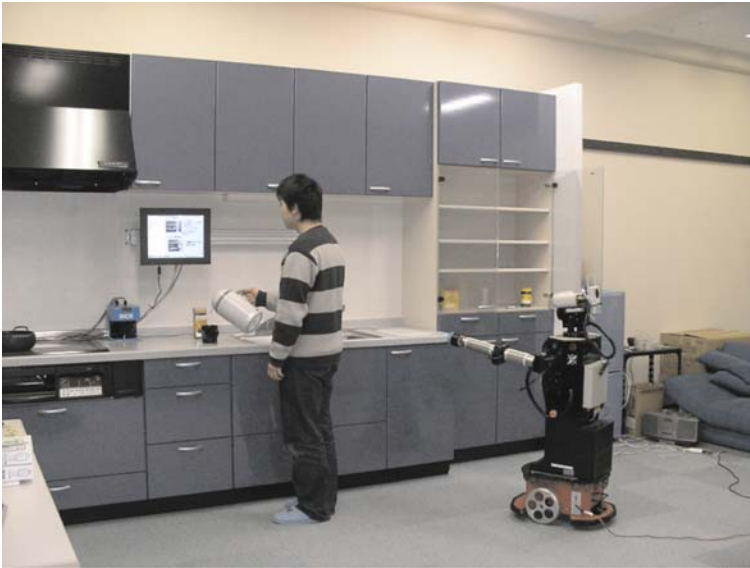
Fig. 4.11 Cooking-support robot recommending a presumed next action to human by voice and gesture.
