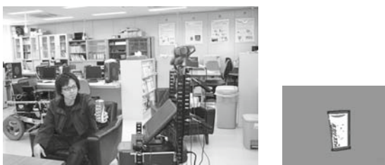
Fig. 11.8 Experimental example 2. When the user said, “Get that,” while pointing toward the object, the robot recognized the object in the rightmost figure as the one indicated by ‘that’ because it was being pointed at.
