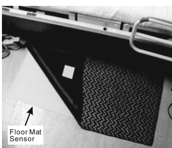
(a) Floor mat sensor at bed side
