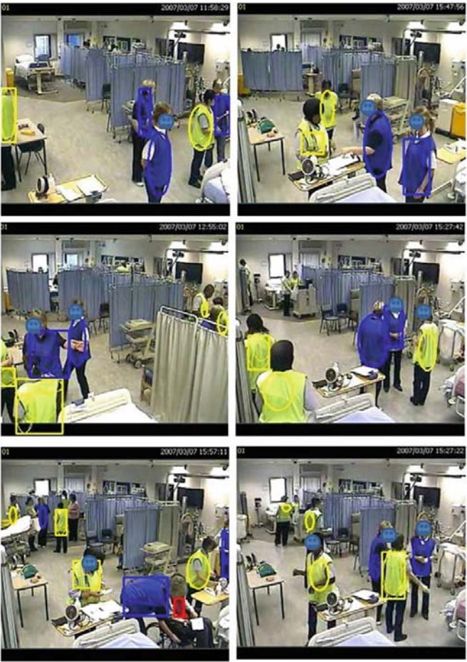
Fig. 7.10 Counting people: In these figures, ellipses represent the original blobs; thick outlines of shapes (rectangles, ellipses) show the existences of individuals; thin outlines of ellipses show the existences of clustered blobs.
