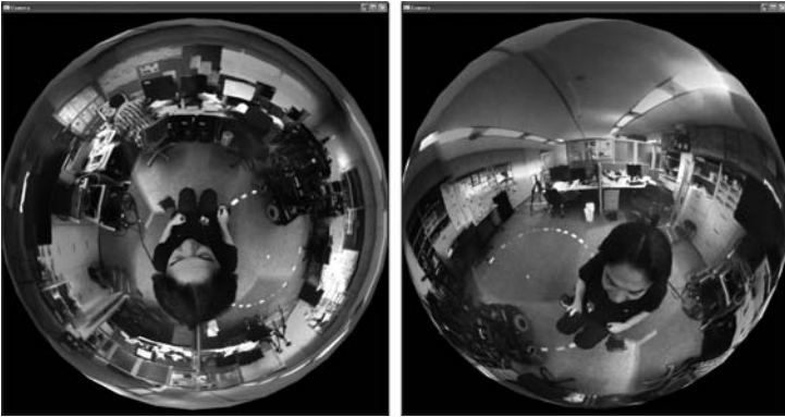
Fig. 8.14 Spherical view of omni-directional images provided by the electric wheelchair.
