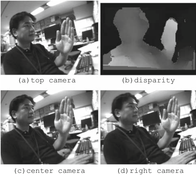
Fig. 8.3 Examples of images captured by the stereo camera unit.
