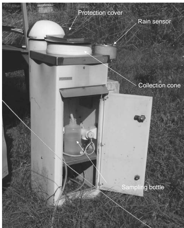
FIGURE 10.2 Wet-only rainwater collector. (From Scheyer, A., PhD thesis, University of Strasbourg, 2004.)
