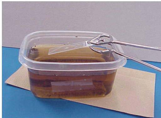
Fig. 9 Touching the capture slide horizontally to the water surface—capturing the AWI biofilm. Reproduced from [2] with permission
