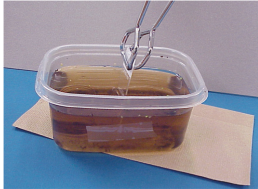
Fig. 10 Removing the captured biofilm vertically, without tearing it. Reproduced from [2] with permission
