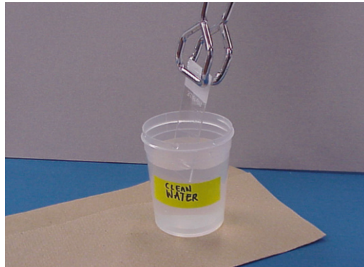
Fig. 11 Rinsing non-AWI microbes away from the biofilm. Reproduced from [2] with permission
