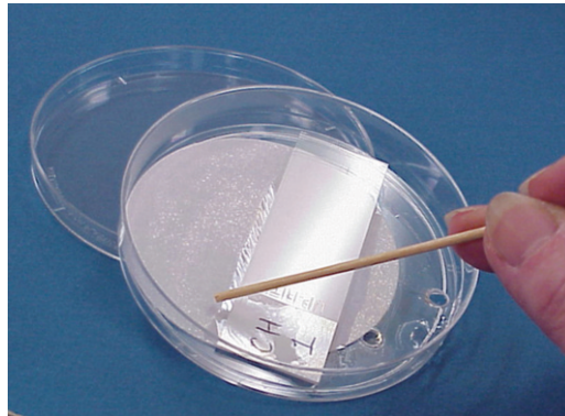
Fig. 6 Removing the slide from the underlying paper. Reproduced from [2] with permission
