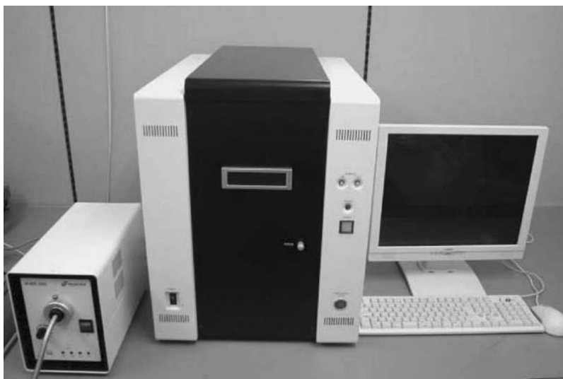
FIGURE 5.5 Outlook of an evanescent-field activated-fluorescence detection-type instrument (SC-Profiler) for lectin microarray. The instrument was developed in the course of the NEDO project designated “SG” (Structural Glycomics) by collaboration with Moritex (Tokyo, Japan).
