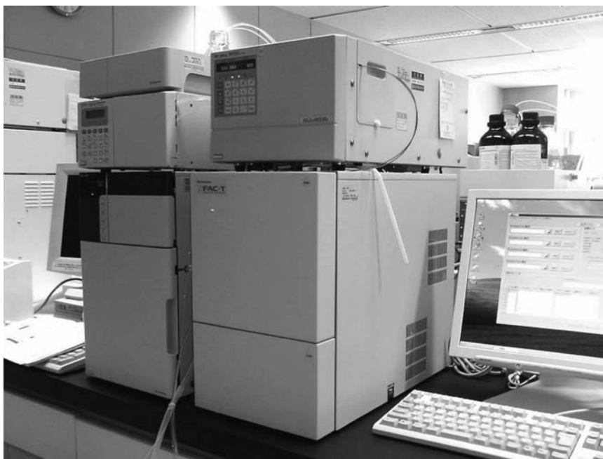
FIGURE 5.1 Outlook of an automated FAC instrument, FAC-T. The instrument was developed in the course of the NEDO project designated “SG” (Structural Glycomics) by collaboration with Shimadzu Corporation (Kyoto, Japan). The FAC-T instrument consists of two isocratic pumps, an autosampling system, a column oven, a pair of miniature capsule-type columns, and a PC workstation. In this system, FAC-T is equipped with a fluorescence detector. For details, see text. (From Nakamura-Tsuruta, S., Uchiyama, N., and Hirabayashi, J., Methods Enzymol. , 415, 311, 2006; Nakamura-Tsuruta, S. et al. In: Nilsson, C.L., Ed., Lectins: Analytical Technologies , Chapter 10, Elsevier, Amsterdam, 2007.)
