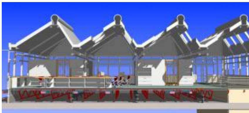
Figure 2: Longitudinal section through the Robert L. Preger Intelligent Workplace at Carnegie Mellon University, which incorporates natural ventilation (cross and stack), daylighting and passive solar heating
