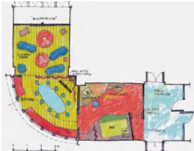
Figure 1. Conceptual design of the floor-plan indicating the comZONES. In the inner black zone the individual can be both seen and heard by the VMC equipment. In outer gray zone the resident might only be seen but not heard. In the surrounding white zone the person can neither be seen or heard. These zones can vary in time and space.
