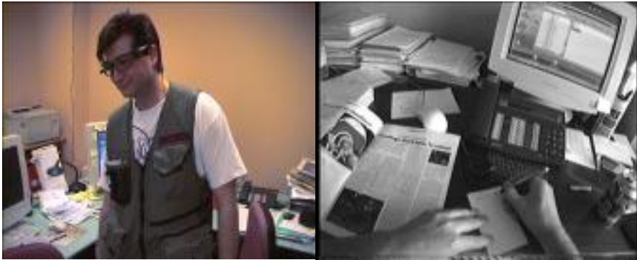
Fig.1 a & b. Left, the first version of the Subcam (1997), with which most observations described here were made. The jacket is convenient, but not very aesthetic and heavy ; the newer versions are nicer and lighter. Right, a picture extracted from a Subcam tape: the subcamer is writing a post-it. Present resolution of 400 lines is insufficient to read what is written in font smaller than 16 on paper or screen, although sufficient for subcamers to remember what they were doing, during debriefing.
