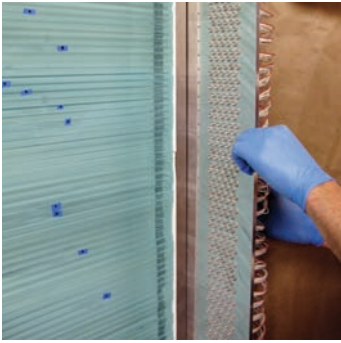
Figure 6.18 LED electronics modules mounted on custom reflector stack to focus LEDs. Blue tape notes where “dimples” are visible that demonstrate that plate glass is not absolutely flat
