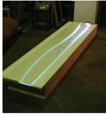
Figure 6.12 Small mock-up prototype to test the curvature of glass, dry stack technique and custom-controllable LED electronics modules
