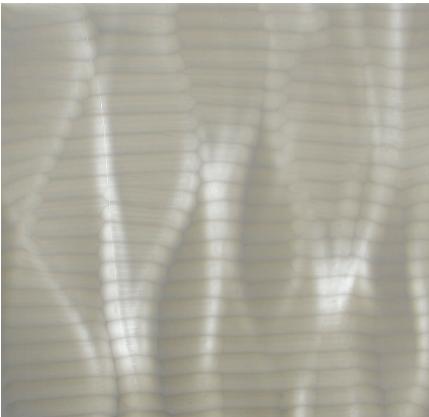
Figure 21.3 Three-axis milled Corian, 12" x 12" x 1/2"
