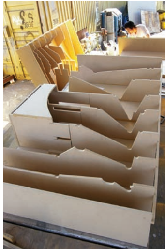
Figure 17.12 Live Wire . Wood jig used for the fabrication of Live Wire
