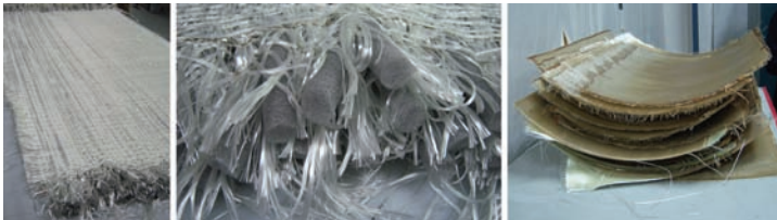
Figure 9.7a–c Three-dimensionally woven fabric and cured panels
