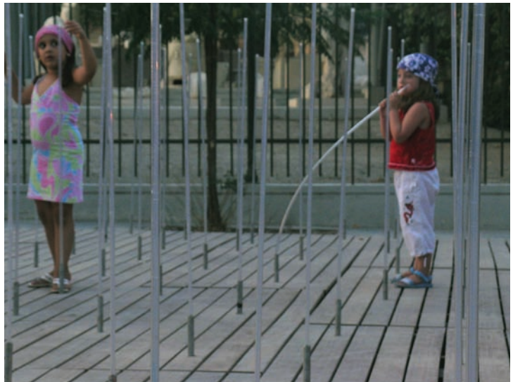
Figure 6.9 Fiber optics housed in polycarbonate tubes allow for flexibility and bending
