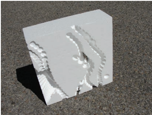
Figure 21.4 Six-axis drilled EPS foam 12" x 12" x 4"
