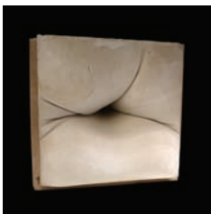
Figure 30.7 First experiment with flexible formworks, MATSYS
