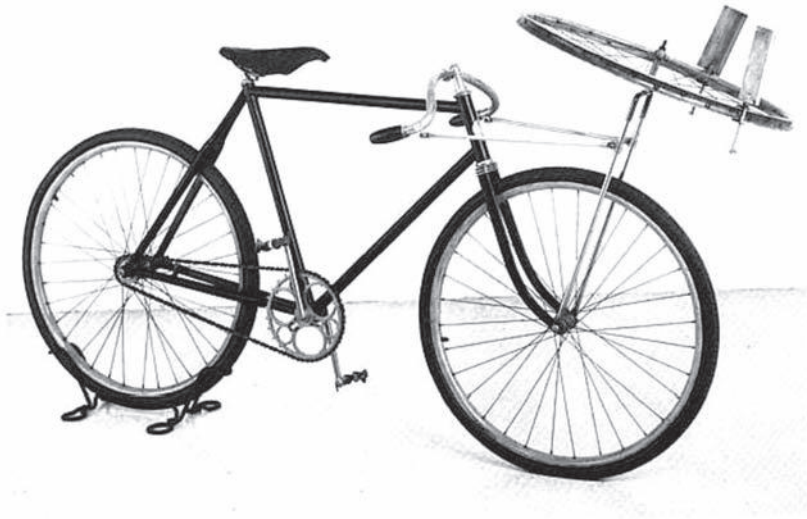
Figure 8.1 Quasi-experimental theory/experiment that led the Wright brothers to both validate their understanding of aerodynamics and debunk years of scientific theories, leading directly to the first manned flights of heavier than air vehicles
