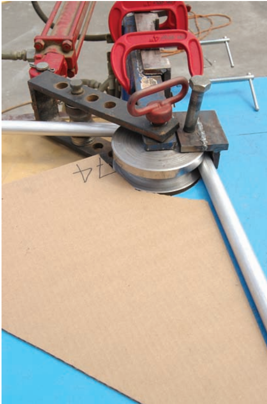
Figure 17.9 Live Wire . A custom die was milled for a hydraulic tube bender to create a 2" radius bend for the 1" diameter aluminum tubes. Also shown is a cardboard template used to determine the exact angle of the bend
