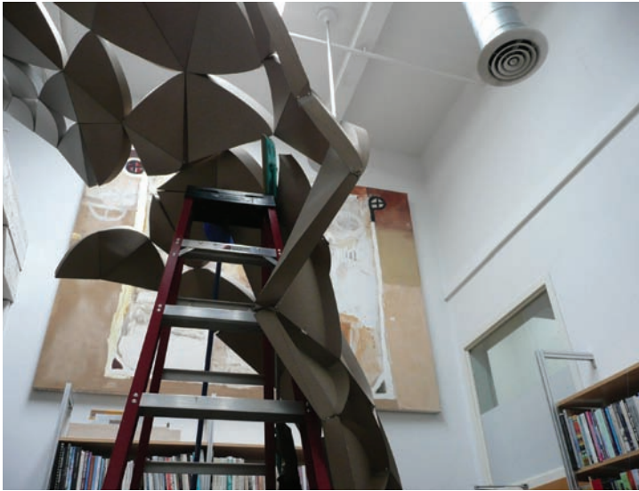
Figure 2.18 Chipboard vault mock-up structural failure
