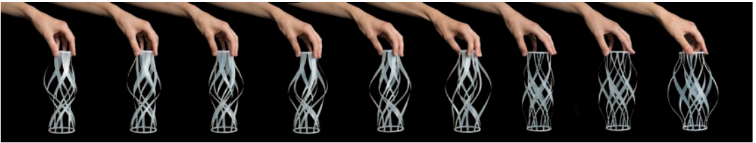
Figure 6.41 Study model of twisting weave under various rotations, compression, and torque
