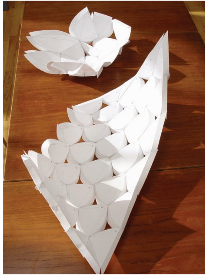
Figure 2.3 Delaunay triangulated and diagrid paper prototype assemblies
