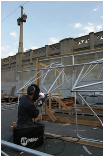
Figure 17.14 Pendulum Plane . An armature was constructed to test the movement of each unit and to ensure accurate operation. Once the units were placed in the armature, the pivoting flaps were then welded on
