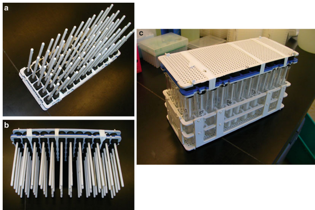
Fig. 3. Custom-made stir-rod array used for thoroughly mixing diluted samples before analysis. (a) Top view. (b) Side view. (c) Stir-rod array dipped in 10 % nitric acid in tube set during storage.
