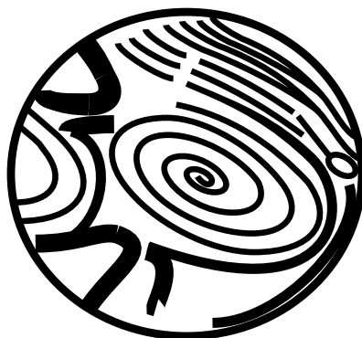
Figure II.1 The 2D patterns formed by adsorbed CO and O on Pt surfaces. (From Ertl, G., Science , 254 , 1750, 1986.)
