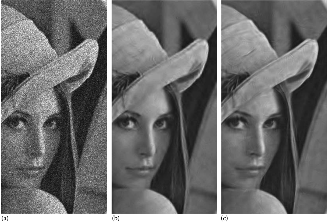
FIGURE 25.25 Denoising results using Lenna (a) Image with additive white Gaussian noise with \sigma = 22.5 . (b) Denoised image using the UDWT. (c) Denoised image using Bamberger pyramids.
