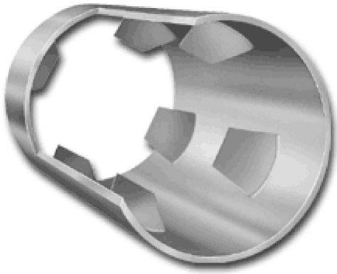
Figure 10.25. The Kenics vortex tab mixer (HEV).
