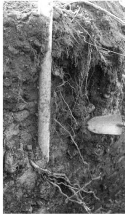
b) Roots concentrated around the Neutron Probe access tube
