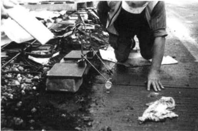
Photograph 4, HA 6/80 dial gauge testing
