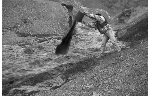
Figure 6.9 Slug injection of a dye tracer into a turbulent flash flood of a small arid stream.
