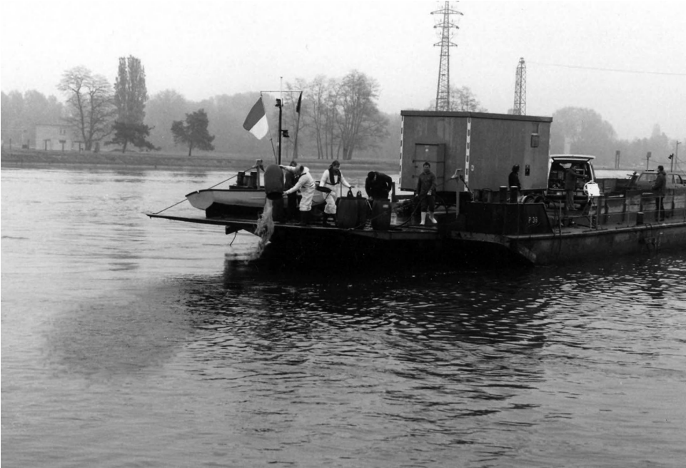
Figure 7.23 Tracer injection into the Rhine downstream of Basel.
