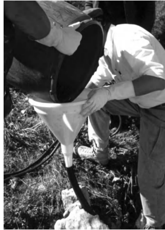
Figure 6.5 Injection of a tracer into a well by means of a pump and a hose.
