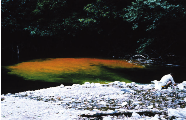
Plate 6a: Situation 10.27 a.m.: The portion of the traced water contained in the right vortex reaches the right bank leading to the start of the left rotation along the right bank.
