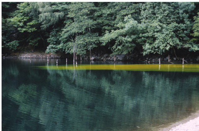
Plate 6c: Situation 11.10 a.m.: Part of the tracer cloud in the left rotation which will pass the lake counter clockwise along the banks and end in a complete mixing within the lake due to complex vortices, diffusion and dispersion processes.
