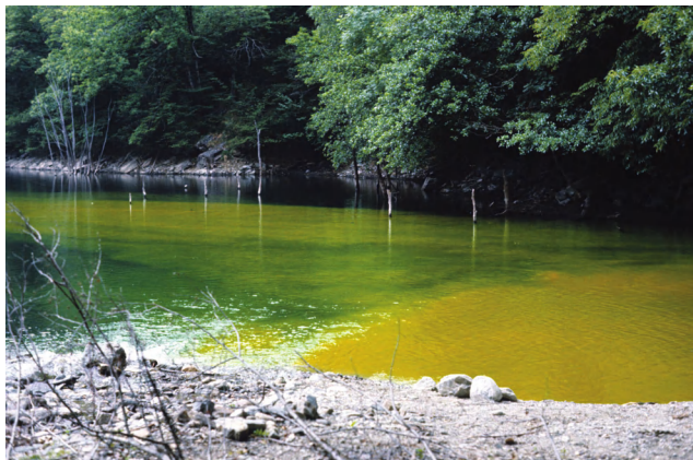
Plate 6b: Situation 10.40 a.m.: The bay right hand of the injection is filled up with traced water (right vortex) and successively the traced water flows along the right bank and continues over into the left rotation.
