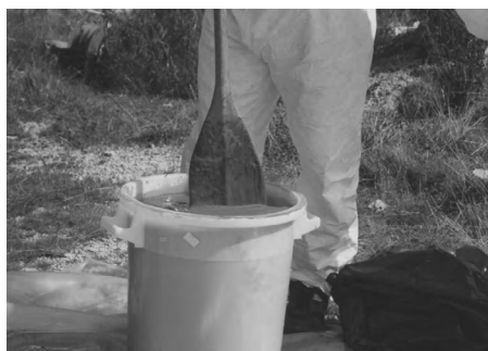
Figure 6.4 Preparation of a concentrated fluorescence tracer solution and the required precautionary measures.
