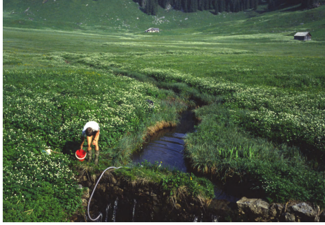
Plate 4a: Typical sediment subcatchment in the recharge area of Churfirsten Mountains (CP3a). The loamy sediment-soil cover (barely vulnerable) drains the water by superficial channels discharging into karst ponors (sinkholes), thus leading to (very) a high vulnerability of the subcatchment.
