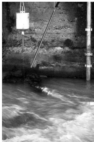
Figure 6.10 Constant rate tracer injection of a fluorescent tracer using a Mariotte bottle.
