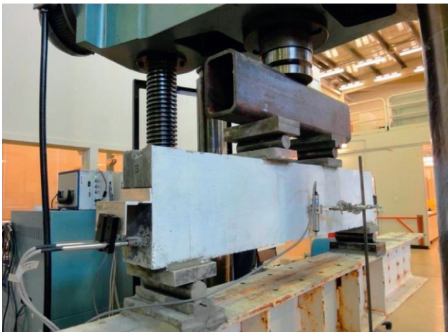
Figure 14.4 Setup of beam-bending test.
