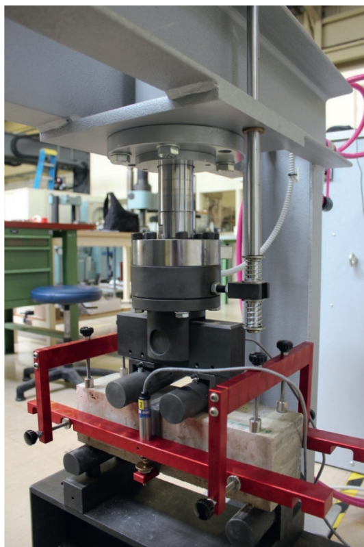
Figure 7.2 Setup of the four-point bending test.
