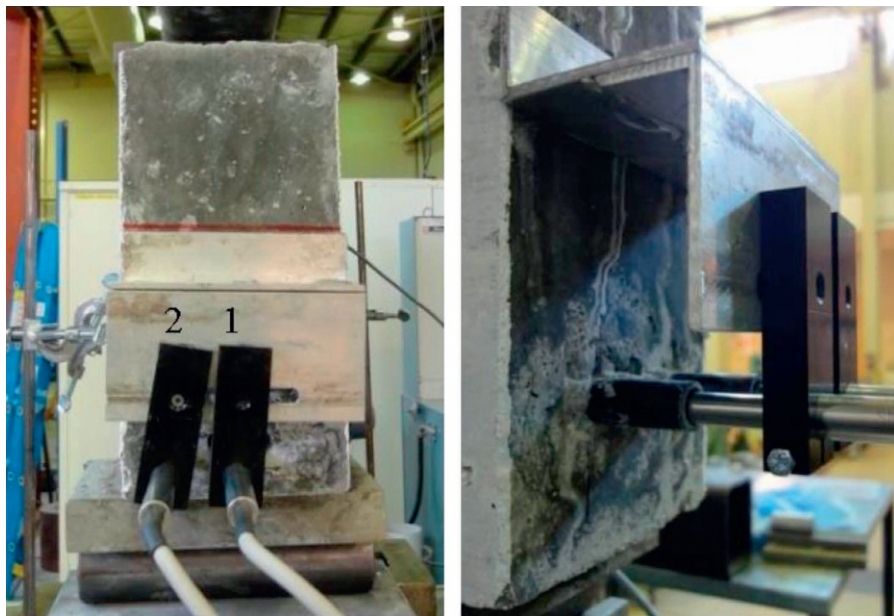
Figure 14.5 Arrangement of LVDTs for bending test.
