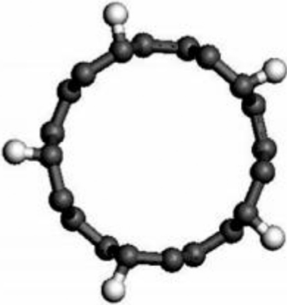
Figure 13.1 Cross section of CNT functionalized by H atoms.
