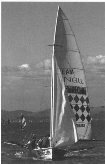
Both sails and fabric roofs must be held taut over supporting structures in order to avoid wind flutter.
