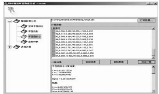
Figure 4. The program of deformation monitoring system of the circular tunnel cross section.
