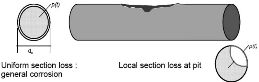
Figure 5. Section loss due to uniform and pitting corrosion.
