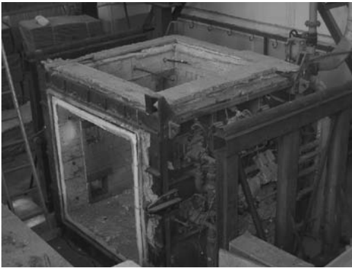
Figure 5. Standing / horizontal fireproof test furnace (1.15 m × 1.15 m).
