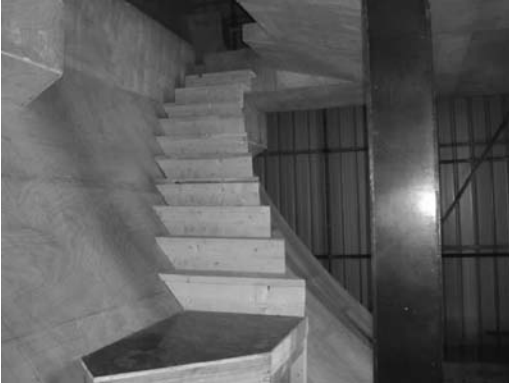
Figure 12. Wooden prototype of escape stairs.
