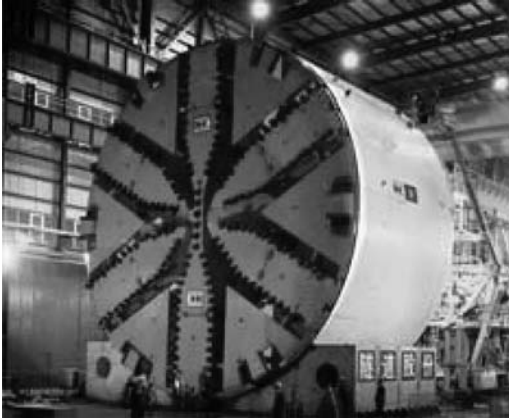
Figure 2. Shield machine used in Shanghai Yangtze River Tunnel.
