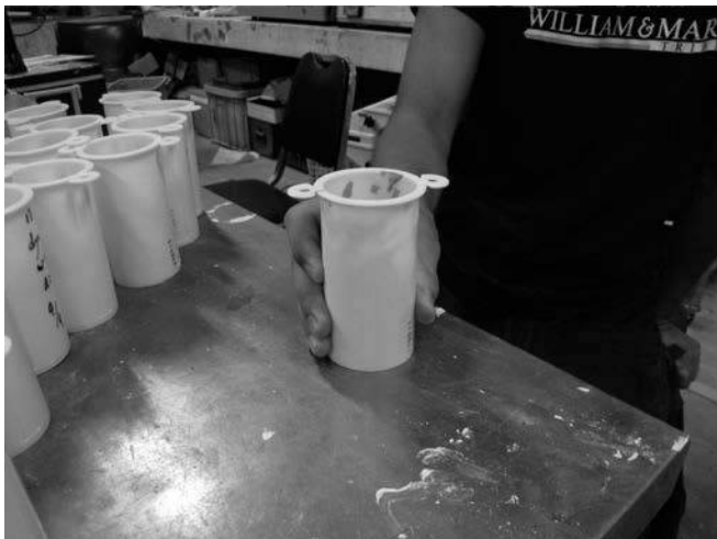
Figure A.4 Tapping technique in molding procedure, used to release trapped air bubbles.
