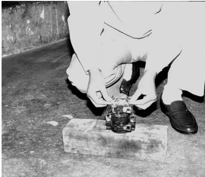
Figure A.5 Sealing the soil sample in the mold with plastic film.
