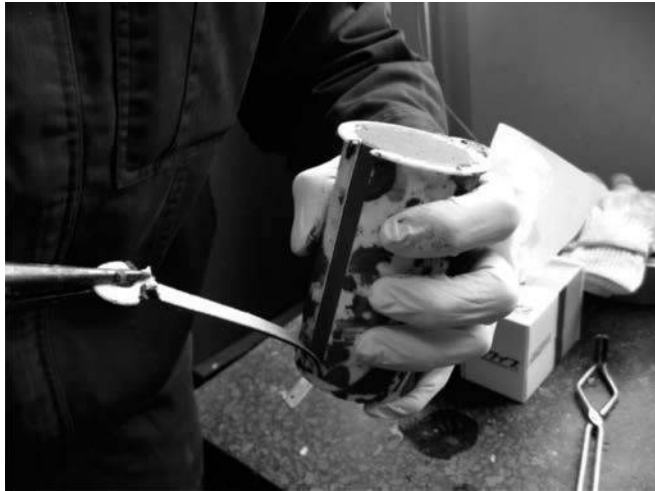
Figure A.7 Removal of a specimen of stabilized soil from a lightweight plastic mold by splitting it along pre-processed slits.
