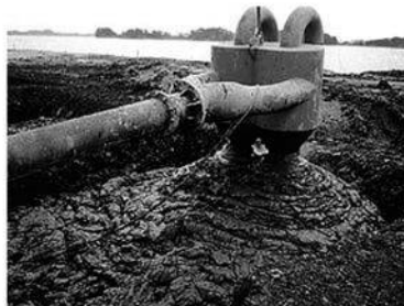
(c) Air pressure release cyclone type placement machine.
