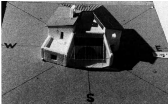
Fig. 4. Heliodon study of model - 2pm June 21st
