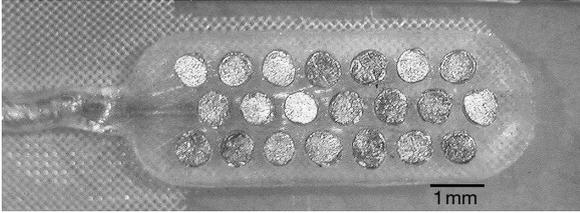
**Fig. 1.** An array of 21 platinum disc electrodes used in the present version of the ABI manufactured by Cochlear Ltd. The platinum electrodes are mounted on a carrier of silicone elastomer.
