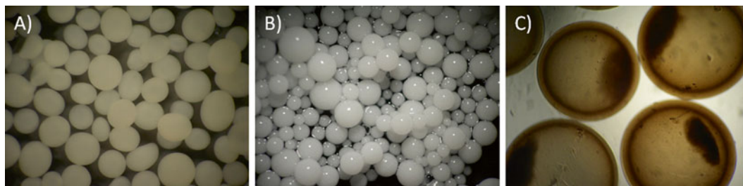
Fig. 4 Final form of the biocatalyst: entrapped and encapsulated IBs. (a) Entrapped IBs- EcSAA in alginate beads, 5 min hardened with 0.5 % glutaraldehyde; the beads became slightly yellow. (b) Entrapped IBs- EcPPK in agar obtained by dispersing and cooling in the vegetable oil. (c) Encapsulated IBs- TvDAO ; the IBs sediment in liquefied core inside the capsules
