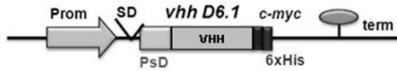
Fig. 1 Schematic representation of VHH D6.1 expression cassettes. SD Shine Dalgarno sequence, Prom psychrophilic L-malate inducible promoter, term psychrophilic terminator, PsD PhDsbA signal peptide
