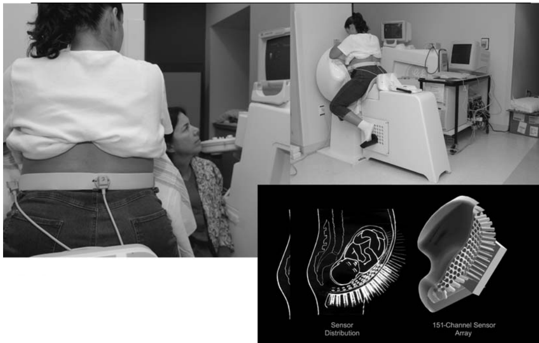
Figure 5. Device used to collect magnetic fields generated during electrical activation of any organ. In this instance, magnetoencephalography is used to monitor fetal brain activity non-invasively. From Curtis L. Lowry Jr., University of Arkansas Medical Center.
