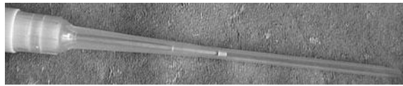
Fig. 1. Example of a positive displacement pipette with a piston in the pipette tip.
