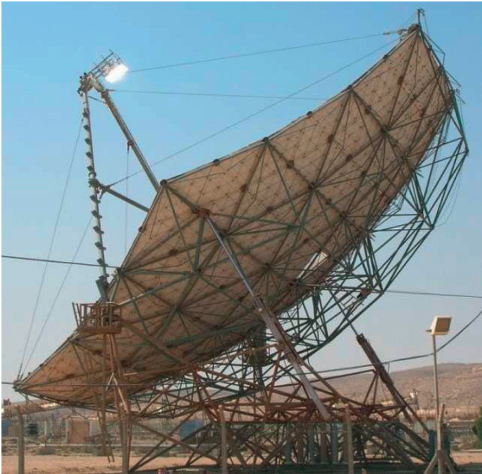
Figure 27.3: CPV cell module exposed at 1000X at the 400 m 2 PETAL solar dish test facility in Sede Boqer, Israel. Source: Photo by David Faiman.
