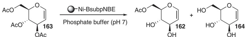
**Scheme 44** The continuous flow ester hydrolysis achieved using a flow reactor containing immobilized His<sub>6</sub>-tag BsubpNBE.
