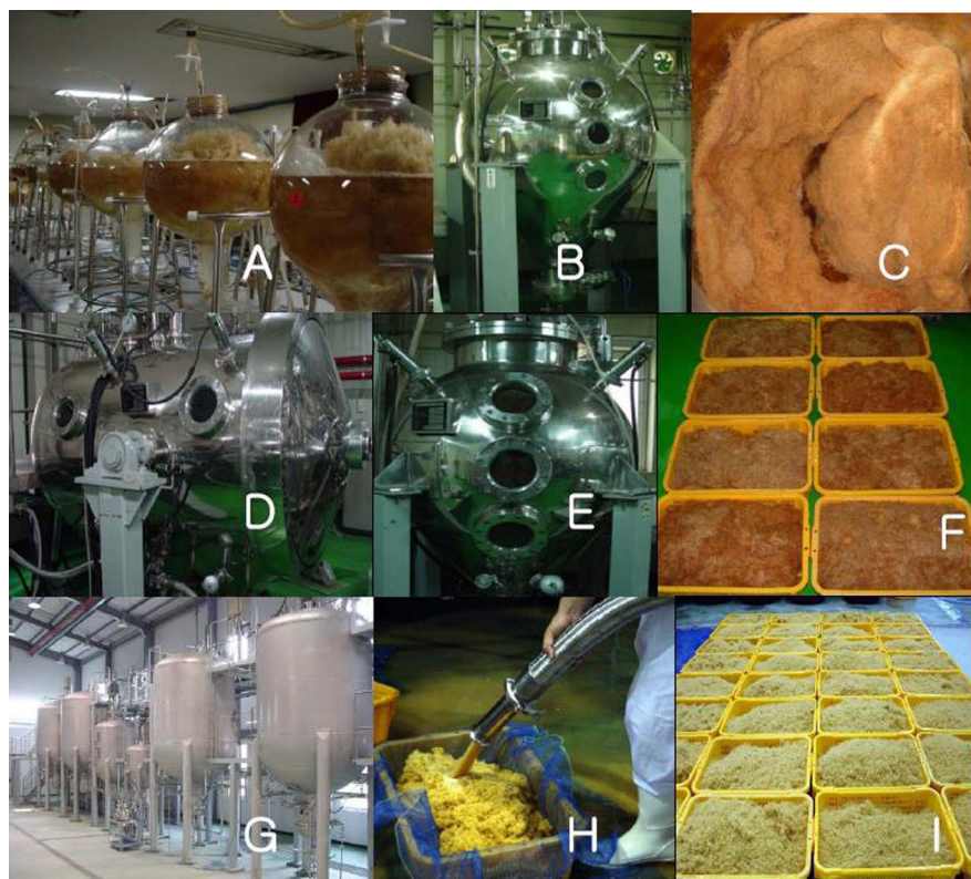
Figure 6.2 Cultivation of adventitious roots in liquid-phase air-lift bioreactors (20–10 000 L). Adventitious roots of Echinacea purpurea : 20 L, 500 L (A and B) and 1000 L (C and D); Hypericum perforatum : 500 L (E and F); Ginseng : 10 000 L (G and I).
