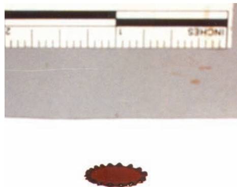
Figure 5.8 Displacement phase in a 90° impact. Note the displacement of the liquid to the rim of the developing stain. All motion up to this point in the collapse is lateral (outward).
