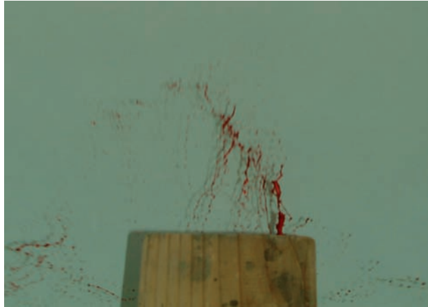
Figure 3.16 Impact spatter radiates out from a central area. In this impact, the drops can be seen ejecting forward along the leading edge ( 350^{\circ} to 20^{\circ} ), to the left ( 270^{\circ} to 290^{\circ} ) and to the right ( 80^{\circ} to 90^{\circ} ).
