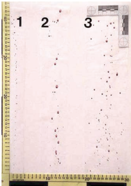
Figure 3.11 Three different cast-off patterns produced by three events. The first was created by swinging an edged weapon, the second with a bat, and the third with a piece of lumber.
