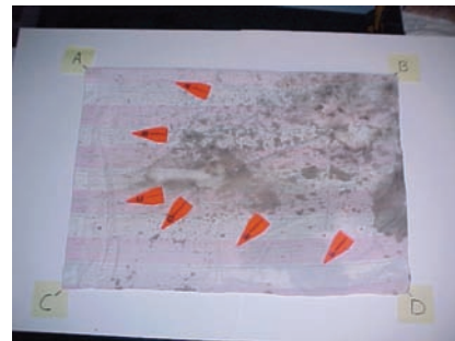
Figure 11.14 Directionality on fabric or cloth is not always a complete lost cause. If we consider the overall pattern, along with the major axis of the involved ellipses, we can still visualize the radiating nature of the spatter pattern, which defines the directionality.
