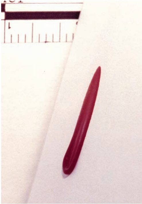
Figure 5.9 Early displacement of a droplet impacting at an acute angle. Note the distinct rim in the forward edge.
