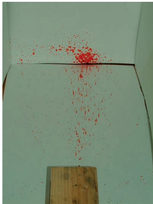
Figure 3.17 The resulting pattern created by the impact observed in Figure 3.16. Note the primary pattern radiates outward from the ejection point. Not all of the stains on the right and left are captured in the photo (they carried to the side walls), but some stains are visible showing the full cone of ejection.
