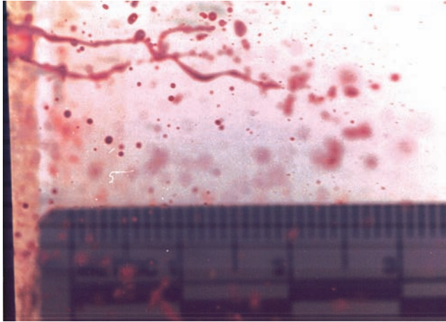
Figure 5.21 Another example of blood displacing due to a force. A mousetrap device to the immediate left of the photograph displaced the blood. As it displaces, spine-like structures are still evident as well as droplets. The spines will degenerate into droplets when the force of displacement overcomes the surface tension and viscosity of the liquid blood in the spine.
