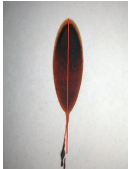
Figure 7.7 The spine associated with elliptical stains will not always align exactly with the directional angle. The red line divides the major axis of the stain and indicates its directionality. Note that the spine shows redirection slightly to the left.
