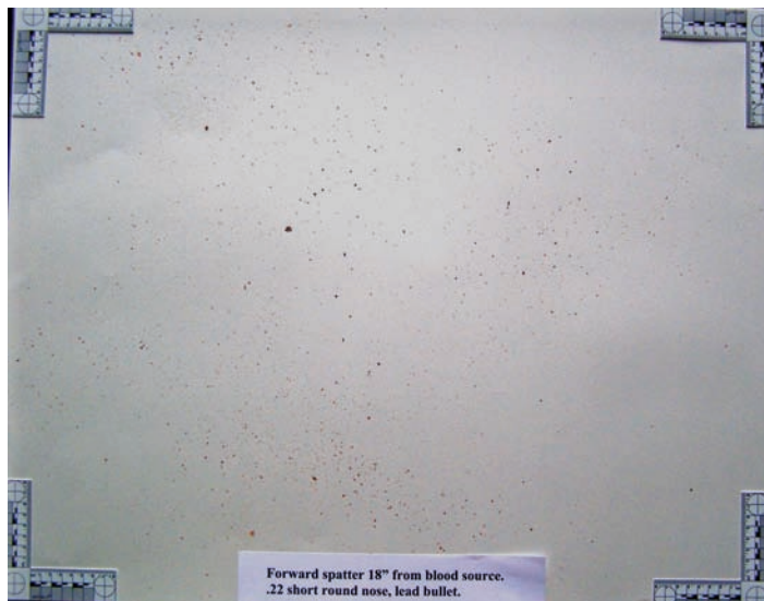
Figure 9.11 This pattern shows the level of dispersion present in a gunshot event when the target was 18 in. from the blood source. The pattern has a more dispersed nature with less of a misting effect.
