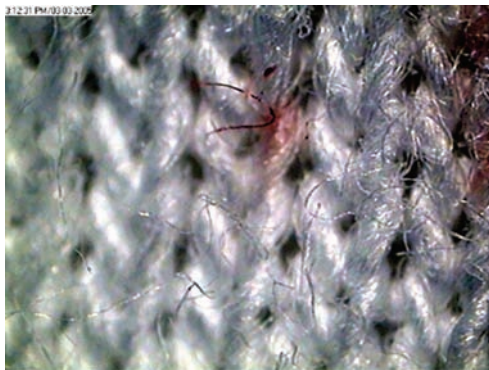
Figure 16.1 A “painted fiber.” After appropriate experimentation (e.g., considering and testing all viable possibilities), it was established that “painted fibers” could be produced by both contact and gunshot. In the context of the case, they served no function in answering which of the two mechanisms was more likely.
