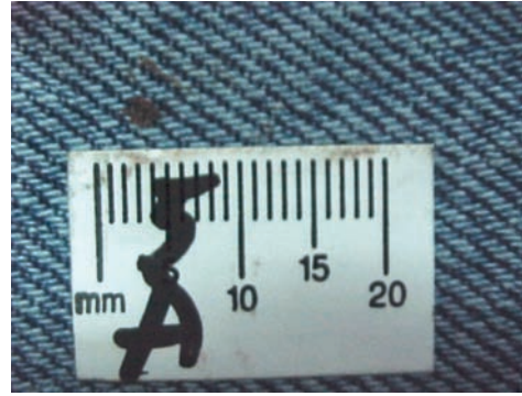
Figure 11.22 A close-up photograph of Stain #5A from Pattern 5 depicted in Figure 11.21. The larger orange label is too big for the macro-photograph, so an additional small millimeter scale is introduced alongside the stain and annotated so the viewer knows which stain they are looking at.
