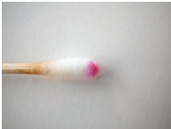
Figure 12.10 A positive phenolphthalein reaction. The swab is moistened with alcohol and then rubbed against the suspected stain. A drop of phenolphthalein solution is placed on the swab, followed by a drop of peroxide. The pink color should develop immediately.
