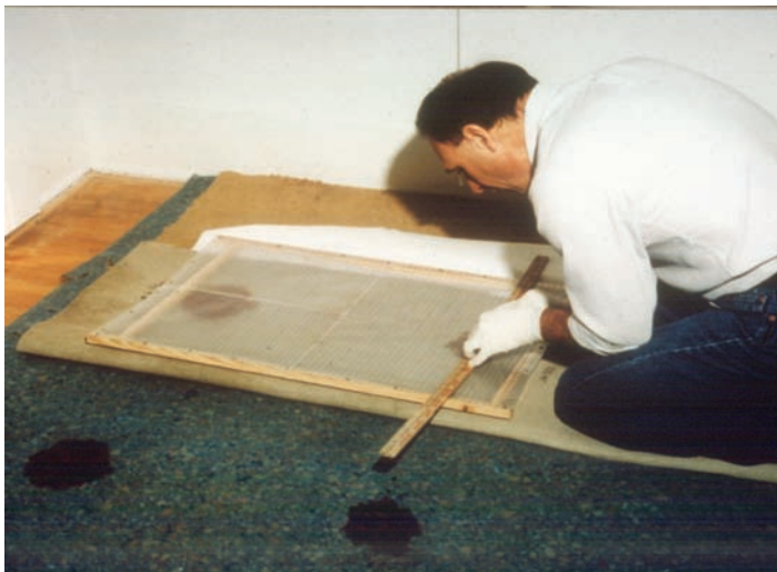
Figure 10.29 The analyst then measures the total area evident in the standards. This figure is compared to the area in the questioned stain. This comparison in correlation to the known volume of blood used to create the standard allows the analyst to estimate roughly the volume of blood in the questioned stain.
