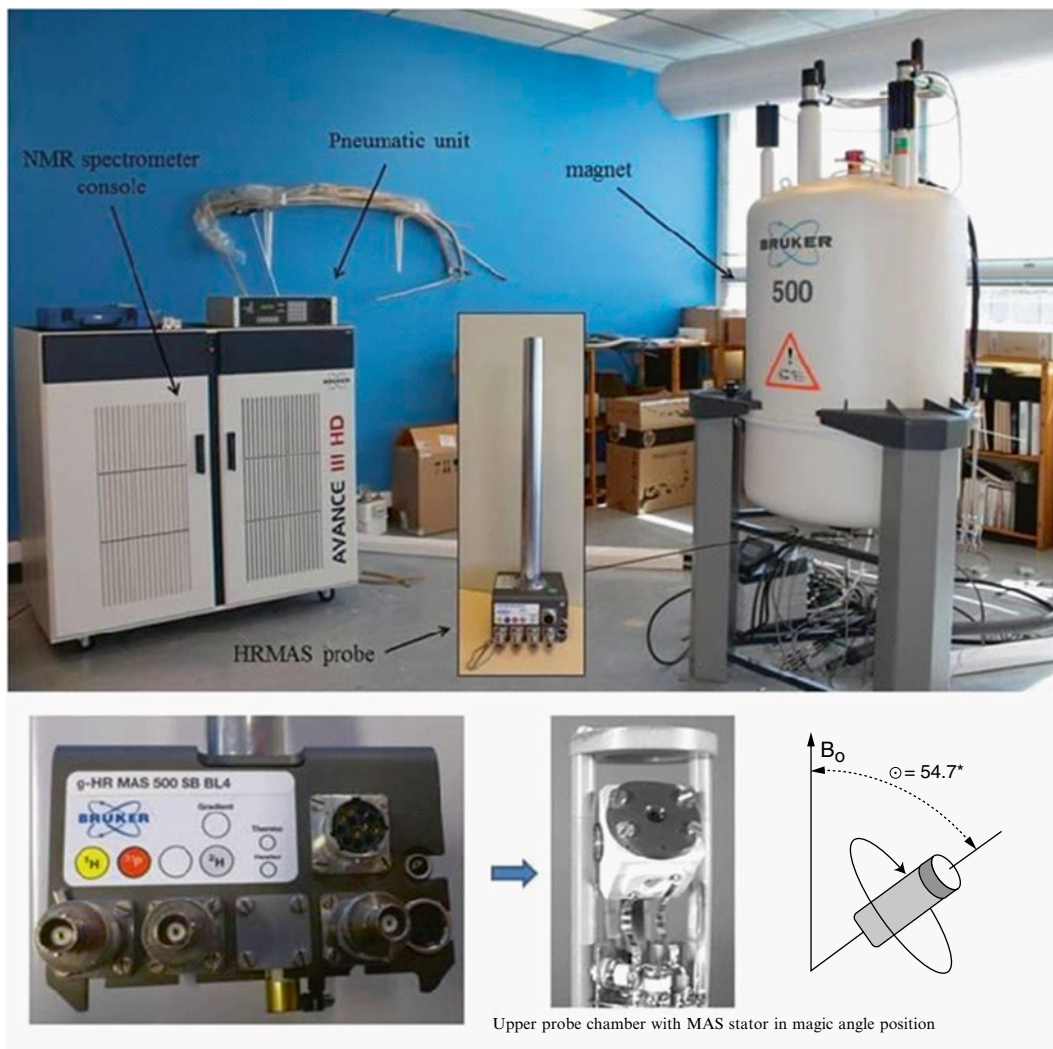
Fig. 1 500 MHz NMR spectrometer (11.7 T) equipped with HRMAS probe
