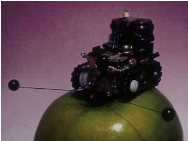
Robotic ant that can act as part of a team. The extending wires are touch sensors.
