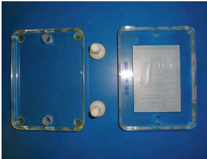
Fig. 4 NC is aligned to the upper part of Miniblotteder® with the reference line parallel to channel 1
