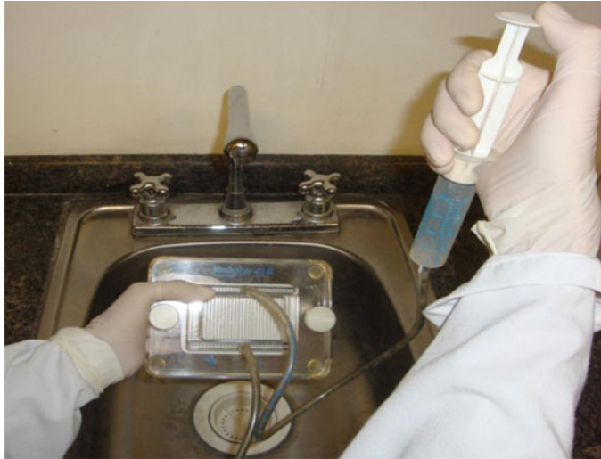
Fig. 11 Antigen excess can also be removed by washing with 40 mL PBST using the manifold provided with the equipment
