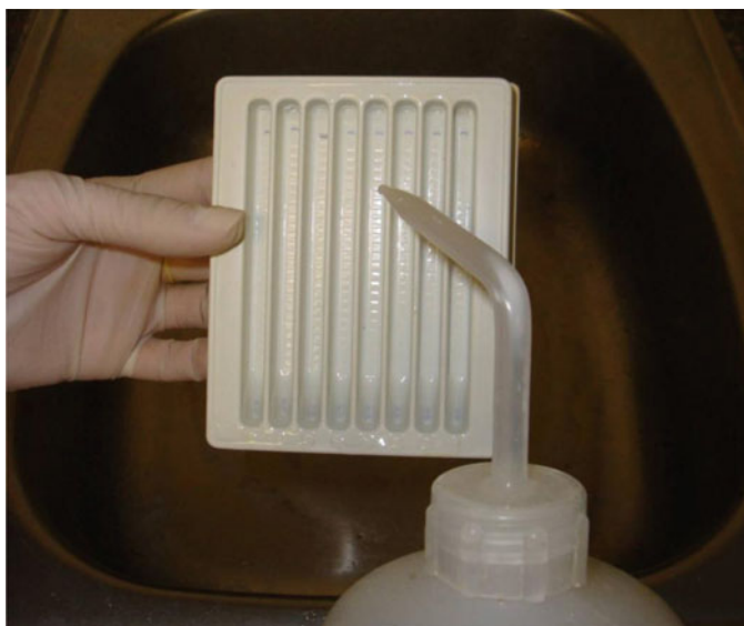
Fig. 18 Strips are washed three to five times for 10 min each, with PBST on a shaker
