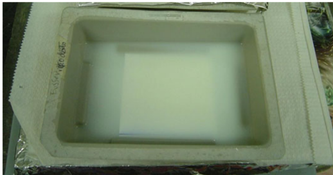
Fig. 12 Blocking is achieved by immersing the NC sheet in 5 % nonfat milk in PBST for 2 h on a shaker
