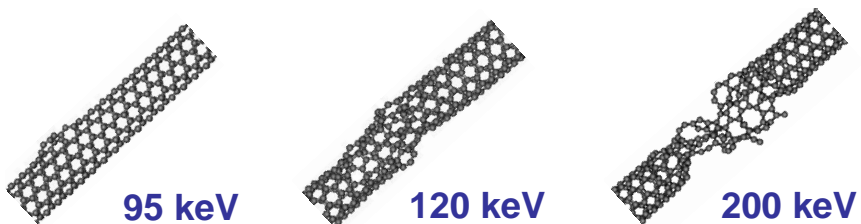
Figure 5. Structures of electron-irradiated (5,5) SWNTs at different electron energies. With increasing electron energy, the irradiation damage became more serious.
