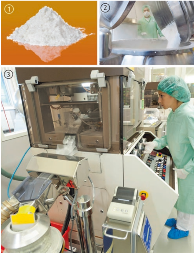
Fig. 2 Bromelain base powder is pressed into tablets. For protection against denaturation bromelain tablets should carry a gastro-resistant coating (pictures from manufacturing facilities kindly provided by B. Roeder, URSAPHARM Arzneimittel GmbH)
