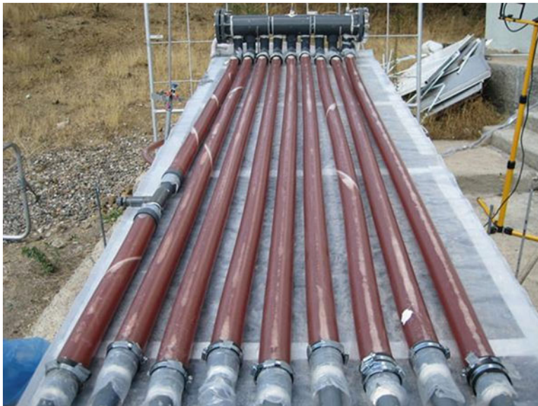
Fig. 11.5. Tubular photo-bioreactor (85 L) operated at METU, Ankara (Reproduced with permission from Boran et al. 2012a).
