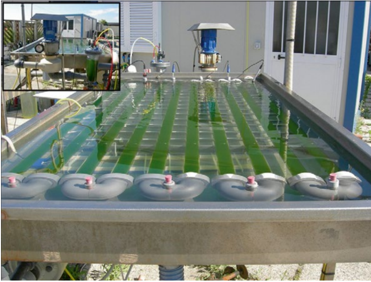
Fig. 13.6. Overview of the 50-L horizontal tubular photobioreactor used for outdoor experiments with C. reinhardtii . Inset: details of the PVC pump and the degasser (Courtesy of Dr. G. Torzillo, ISE, CNR, Florence, Italy).
