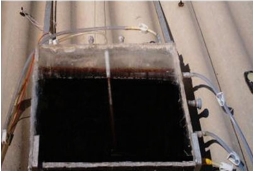
Fig. 11.1. Flat-plate solar bioreactor filled with 4 % (v/v) OMW (Olive Mill Wastewaters) (Middle East Technical University, Ankara).
