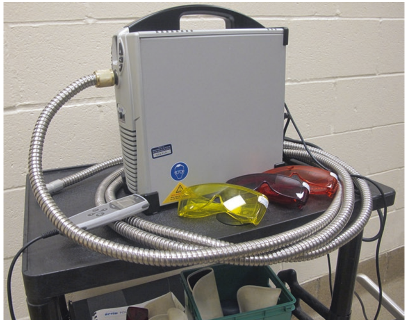
Fig. 3.10 A portable alternate light source and accompanying red, yellow and orange filters
