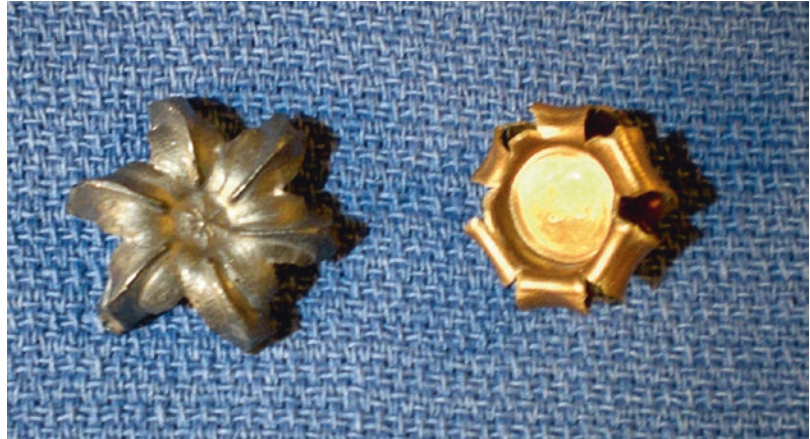
Fig. 7.2 Fired projectile: projectile and semimetal jacket: these may separate in the body both may have evidence of rifling and should be recovered for evidence
