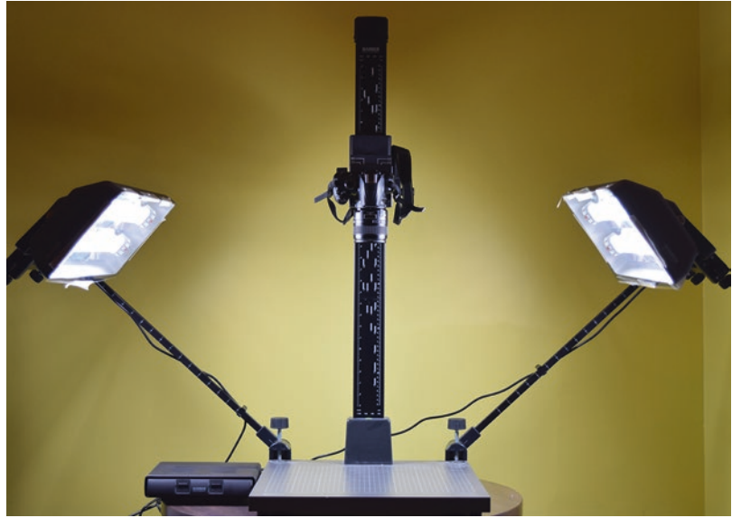
Fig. 3.12 Copy stand with dedicated lighting and digital camera mounted to allow for photography of individual items
