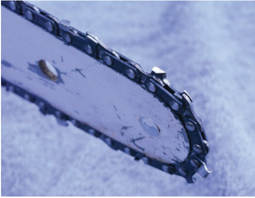
Fig. 6.8 Cutting chain of chainsaw showing individual flat broad vertical and horizontal cutting teeth (Photo courtesy of Dr. Jason Brooks, Penn State University)
