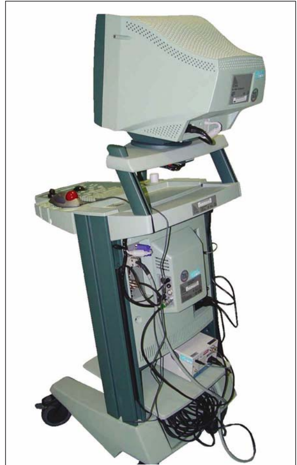
Fig. II.24. New hardware for acquisition, reconstruction, and visualization of three-dimensional ultrasound images
