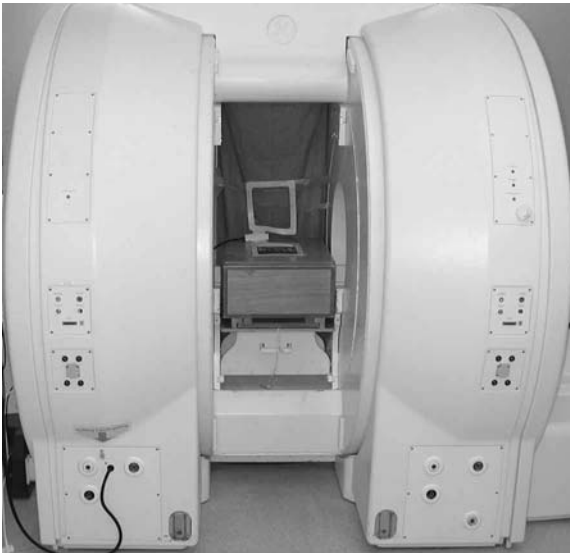
Fig. VI.35. The 0.5 T superconducting, open-configuration magnetic resonance system used for dynamic pelvic examinations. A wooden chair that functions as a toilet allows imaging in the sitting position
