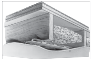
Wood frame—with resilient attachment and mineral wool SAFB
