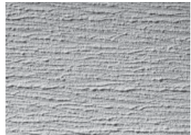
Simple roller-applied texture is obtained with vinyl-base USG Sheetrock® Brand powder, joint compounds. Same products can be used for joint finishing and texturing on job.
