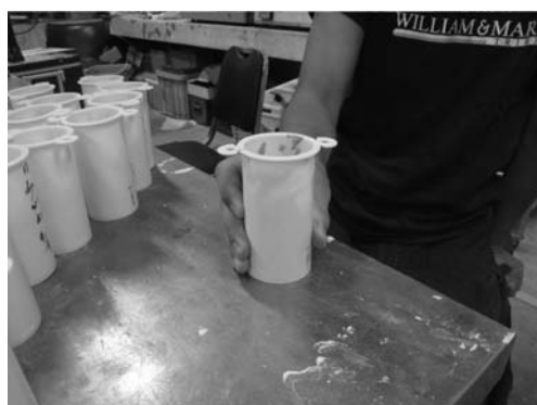
Figure A.4 Tapping technique in molding procedure.
