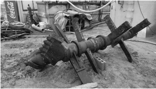
Figure 5.17 Mixing blades and free blade for CDM method for on-land works.
