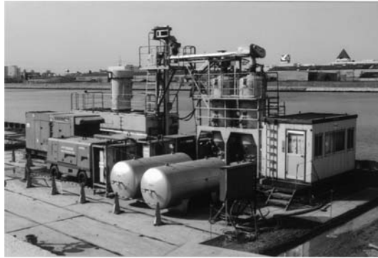
Figure 5.8 Binder Plant for DJM method (by the courtesy of Dry Jet Mixing Association).
