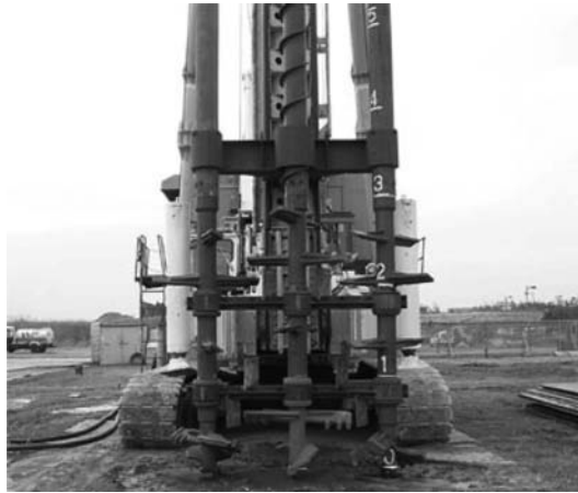
Figure 5.33 Mixing shafts and blades of CDM-Lemni 2/3 machine (by the courtesy of Cement Deep Mixing Method Association).
