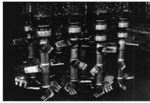
(b) Eight mixing shafts type (Decom 7).
