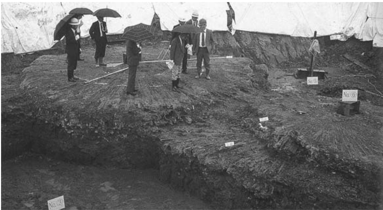
Figure 5.58 Stabilized soil column by Superjet method (Superjet Association, 2011).
