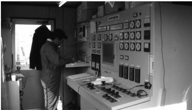
Figure 5.10 Control unit for DJM method (by the courtesy of Dry Jet Mixing Association).
