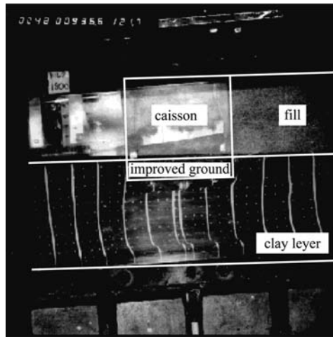
Figure 6.55 Deformation of clay ground between long walls in extrusion failure (Terashi et al. , 1983).
