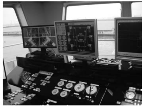
(b) Control desk for operating mixing tools.
