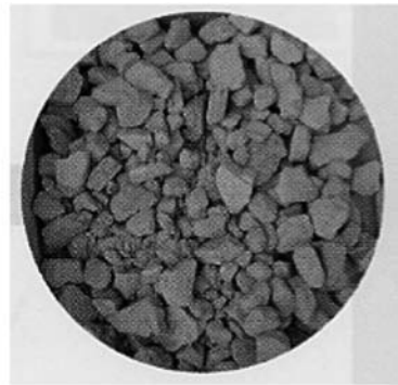
(b) Dewatered Stabilized soil.
