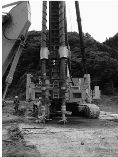
Figure 5.26 Mixing shafts and blades of CDM-LODIC machine (by the courtesy of Cement Deep Mixing Method Association).
