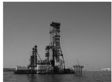
Figure 5.37 CDM barge for in-water works (Cement Deep Mixing Method Association, 1999).
