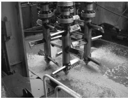
(a) Four mixing shafts type (Pocom 12).
