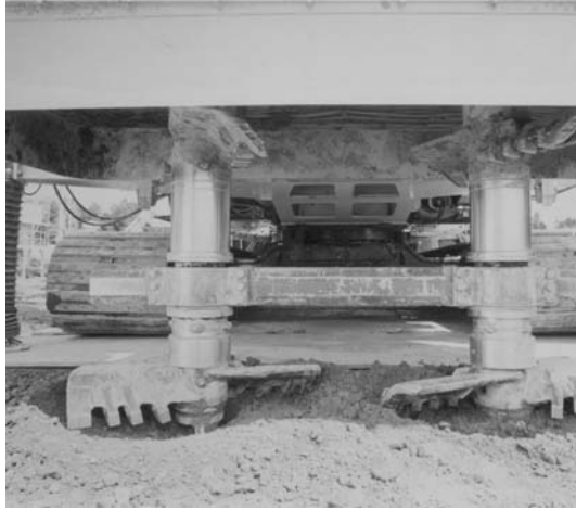
Figure 5.5 Mixing shafts and mixing blades for DJM machine (by the courtesy of Dry Jet Mixing Association).
