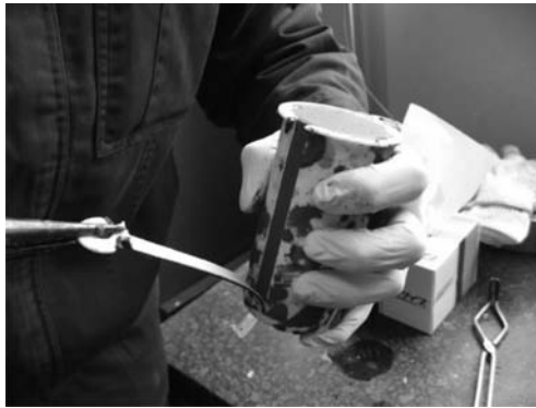
Figure A.7 Removal of specimen by splitting along pre-processed slits of lightweight plastic mold.
