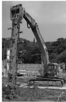
(c) Trencher type (by the courtesy of Power Blender Association).
