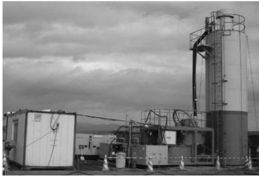
Figure 5.20 Binder silo and pumping unit (by the courtesy of Cement Deep Mixing Method Association).
