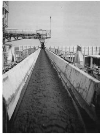
(b) Stabilized soil conveyed to reclaimed site.
