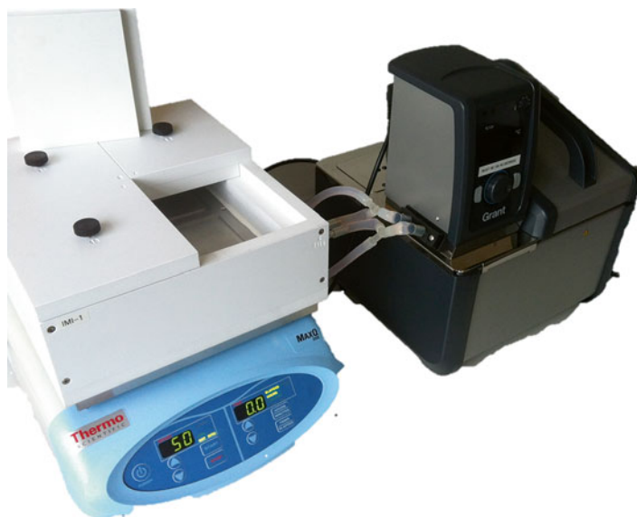
Fig. 3 On-site-constructed incubator on a tempered shaking board
