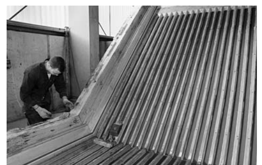
Mould with timber patterning
