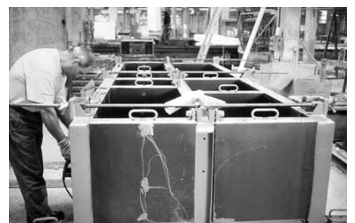
Moulds for precast blocks
