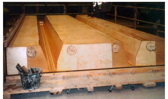
Precast beam mould
