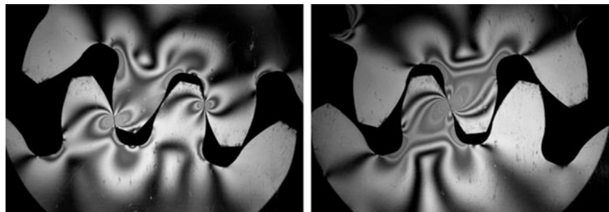
Fig. 6 Photoelasticity study revealing isochromatic stress patterns for double tooth contact (left) and single tooth contact (right) [9]
