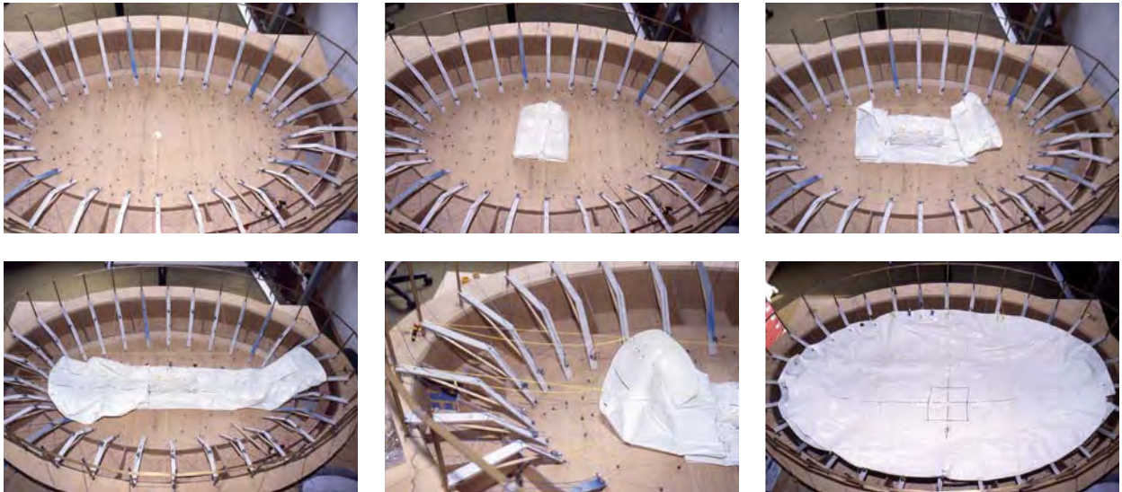
Fig. 154: Erection model for the roofing of the arena at Nimes, France: laying out the pillow
