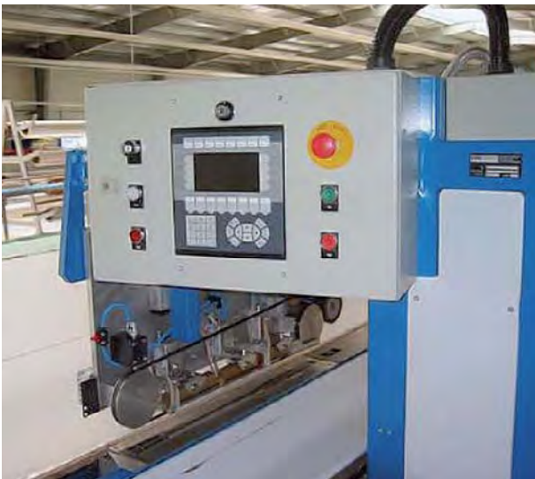
Fig. 116: Welding of ETFE foils
