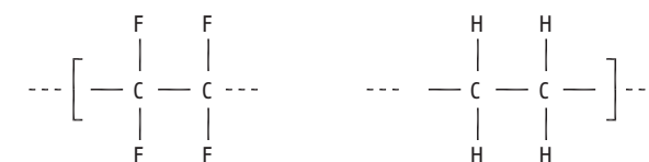
Fig. 58: top: Clear and printed pattern on an ETFE foil bottom: Tetrafluoroethylene / ethylene copolymer (E/TFE)
