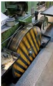
Fig. 12: left: transfer sheave; middle: planetary stranding machine; right: model of a stranding mechanism
