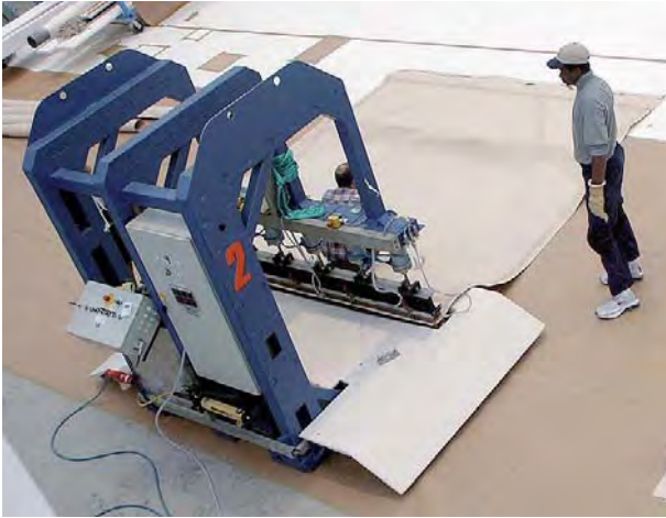
Fig. 115: PTFE heat welding press with a heating beam length of 2 m and a maximum pressure of 7 bar
