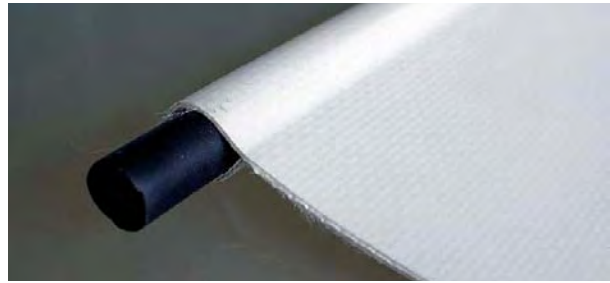
Fig. 43: Welded-in keder in a PES/PVC fabric type 5
