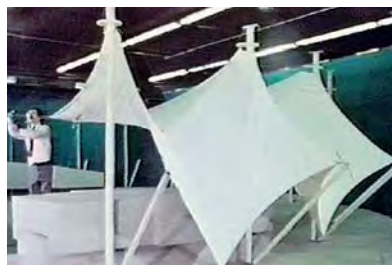
Fig. 157: Model of the erection of the roofing-over of the stands in the stadium of Riyadh, Saudi Arabia
