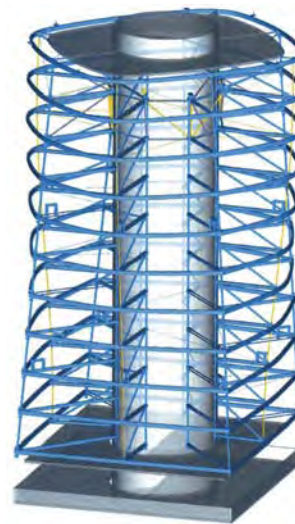
Fig. 228: left: View of a quarter of the steelwork with temporary construction; right: Steel construction around the reinforced concrete core
