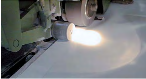
Fig. 112: Grinding off the PVDF paint
