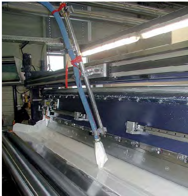
Fig. 52: Top coat with roller knife
