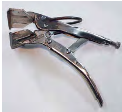
Fig. 192: Longitudinal pulling of a keder rail edge
