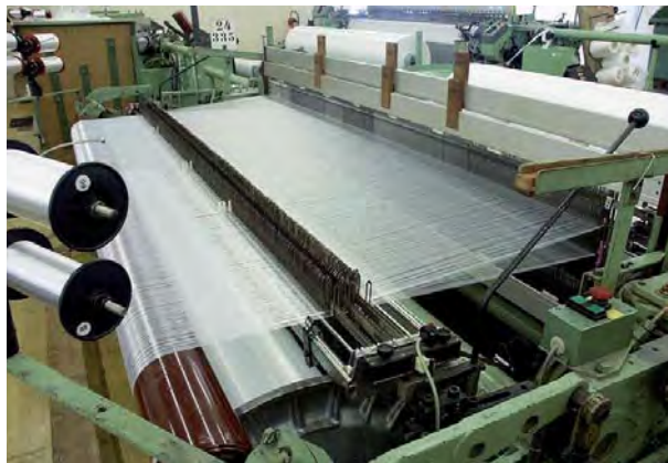
Fig. 48: left: Automatic rapier loom; right: Rapier clamp with weft thread
