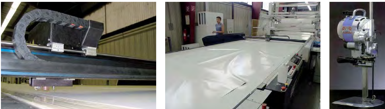
Fig. 108: left, centre: Mechanical cutting machine with round cutter; right: Manual vertical knife machine
