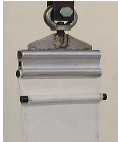
Test of the completed seam
