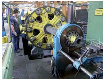
Fig. 12: left: transfer sheave; middle: planetary stranding machine; right: model of a stranding mechanism
