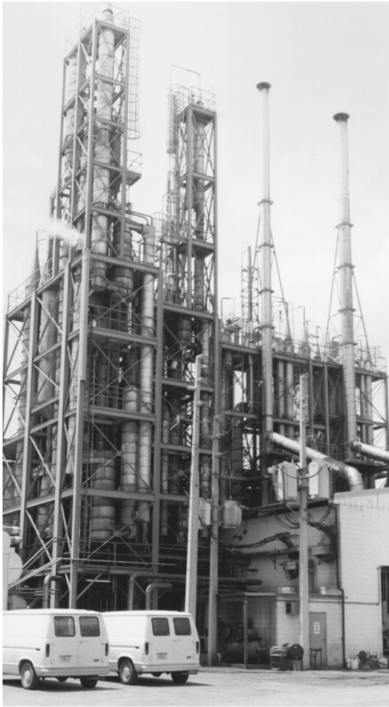
FIGURE 6.5 Typical citrus TASTE evaporator showing stacked design (Courtesy of Alcoma Packing Co., Lake Wales, FL).
