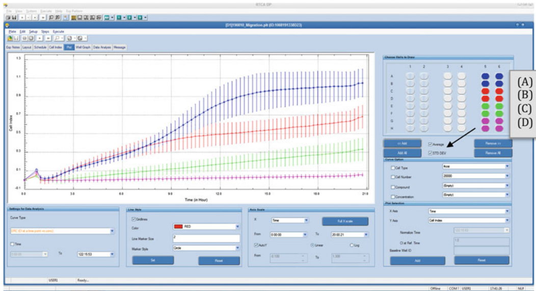
Fig. 4 Example of an experiment visualized using RTCA Software 2.1. This image is a representative plot viewed on the Plot tab on the RTCA Software 2.1. It represents a cellular motility experiment. Wells are highlighted in color and data has been shown as an average of all four wells, with error bars representing the SDEV. These can be chosen by ticking the boxes below the wells ( arrow ). (a) MDA-MB-231 cells untransfected. (b) MDA-MB-231 transfected with non-targeting siRNA. (c) MDA-MB-231 transfected with siRNA against PTK6. (d) Media only
