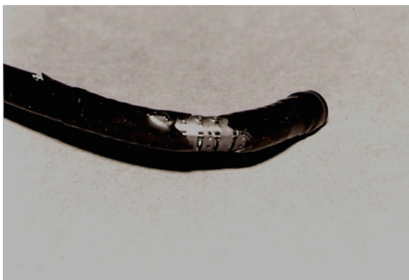
Figure 13-8. Damaged flexible bronchoscope after difficult passage through a tracheostomy tube.
