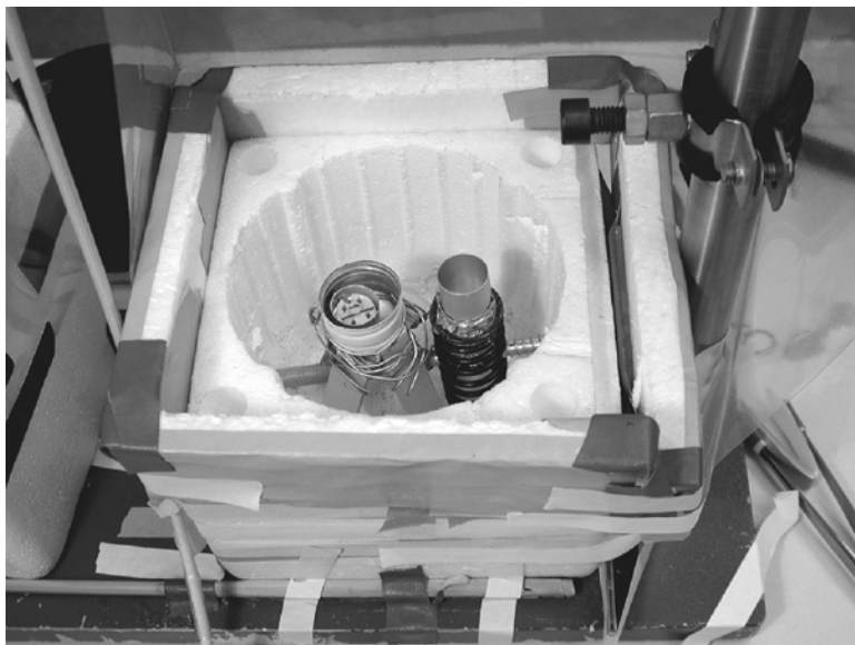
Fig. 2. Bottom part of the plunger device showing the disposition of the ethane pot and the cryo-box.
