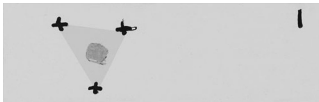
Fig. 3. Tissue section for MALDI Imaging with teach marks for co-registration. Three teach marks are needed for co-registration. In order to reduce the offset to a minimum, the teach marks should be the corners of a triangle covering the tissue section as displayed here in grey.
