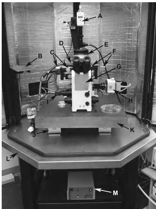
Fig. 2. MFP-3D-BIO AFM setup as configured in our laboratory for macromolecular and cell biology applications includes (a) Top View camera for probe viewing and alignment; (b) MFP-3D-BIO stainless steel platform for mounting cantilever holder on head; (c) optical ( x,y ) alignment controls which move the entire base plate to translate the cantilever and specimen to field of view with bottom view cameras via objectives; (d) x,y scanner; (e) MFP-3D-BIO Head; (f) sample ( x,y ) alignment controls which move the sample relative to the cantilever; (g) IX71 Olympus inverted optical microscope; (h) Hamamatsu video camera for highest resolution viewing and recording; (i) Composite camera for lower resolution viewing and image capture; (j) isolation module ( \times 2 ); (k) granite slab; (l) TMC BCH-45 acoustic enclosure platform; and (m) vibration isolation electronics controller. The ARC2 with Hamster, Fiber-Lite, Hamamatsu, X-cite, and heater controllers are not shown.
