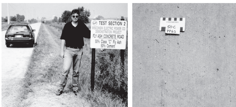
Figure 9.23 (See color insert.) The author examines a slipformed concrete pavement with 50% Class C fly ash after exposure to de-icing salts over six winters.
