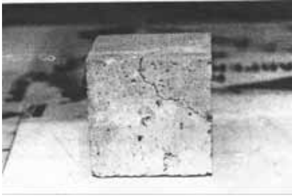
Figure 4.21. Limestone elemental sulfur concrete sample after 14 days of water immersion (adapted from Abdel Jawad and Qudah, 1994).
