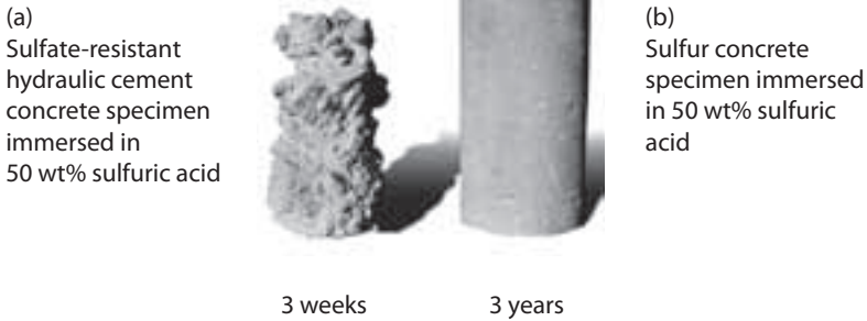
Figure 6.1. Acid effect on sulfate-resistant hydraulic cement concrete and sulfur concrete (adapted from Vroom, 1998).
