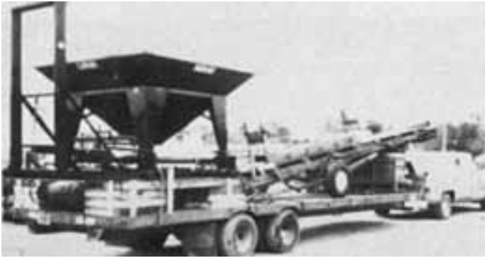
Figure 7.11b. Weigh-hopper, scale and conveyor for the preparation of sulfur concrete mix (Pickard, 1985).
