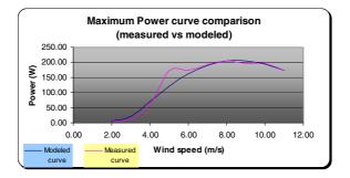
Fig. 7. Comparison of modeled and measured MPPT for wind turbine
