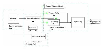
Fig. 2. Function diagram of an energy harvester system
