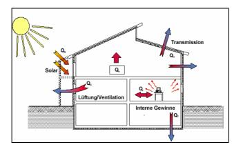
Fig. 8. Heat balance of a building [3]
