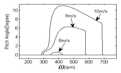
Fig. 7. Pitch angle-Speed curve in Pitch angle control mode for different wind speed
