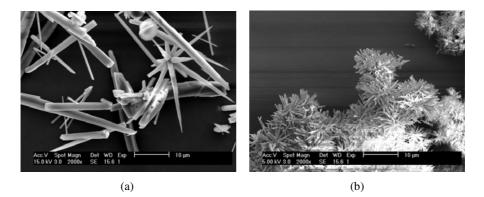
**Fig. 2.** The SEM analysis of crystals collected from the heater cover (stainless steel surface) after the scaling test (a) control (300 mg.l<sup>-1</sup> as CaCO<sub>3</sub>, 42°C) and (b) zinc dosed experiment (300 mg.l<sup>-1</sup> as CaCO<sub>3</sub>, 42°C, 5 mg.l<sup>-1</sup> Zn<sup>2+</sup>)
