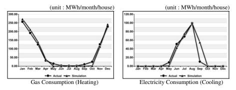
Fig. 1. Comparison of Actual Energy Consumption and Simulation Result
