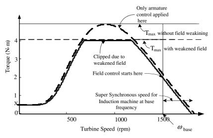
Fig. 3. Torque-Speed characteristics of Wind Turbine Emulator
