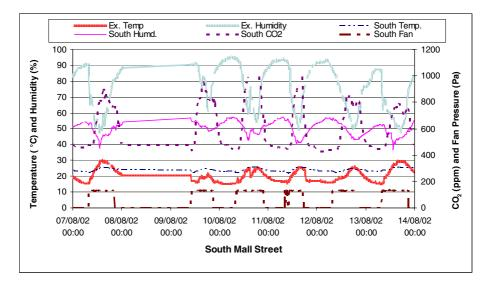
Fig. 3. Measured indoor air quality parameters and fan pressure in the centre of the south mall street
