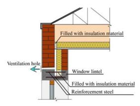
Fig. 6. The connection fabric between exterior wall and roof
