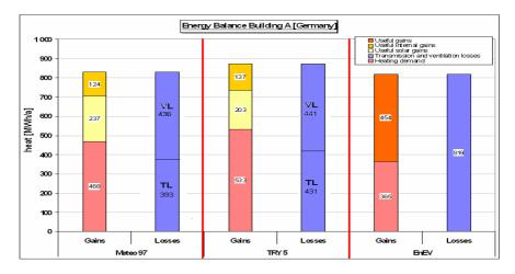
Fig. 10. Energy balance of the building with weather data of Würzburg
