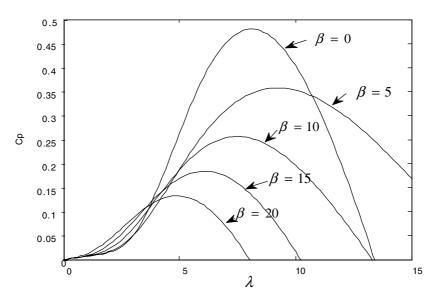
**Fig. 1.** Cp- $\lambda$  curve for various pitch angles
