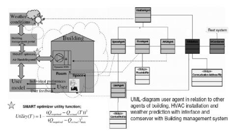
Fig. 5. Conceptual framework SMART with UML-diagram, individual adjustments/energy demands and utility function (Hommelberg 2005)
