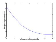
Fig. 5. The effect of increasing the number of turbines in one step ahead predictions of wind speed over average percentage error
