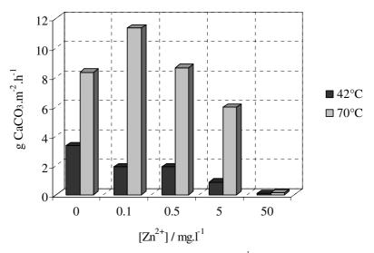
**Fig. 1.** Effect of zinc dosing on CaCO<sub>3</sub> scaling rate (300 mg.l<sup>-1</sup> as CaCO<sub>3</sub>, stainless steel surface at  $42^{\circ}$ C (10 repeats) and 70°C (5 repeats).
