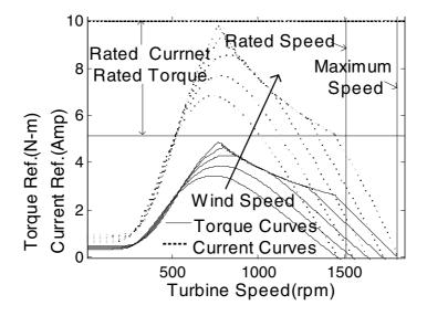
Fig. 8. Reference Current-Speed and Reference Torque-Speed curve for WTE
