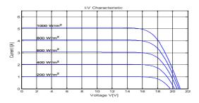
Fig. 1. I-V characteristics with insulation variations and constant cell temperature
