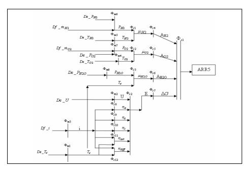
Fig. 7. Oriented graph for chemical part of fuel cell
