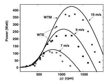
Fig. 9. Experimental Results: Comparison of Power-Speed characteristics obtained using WTM and WTE
