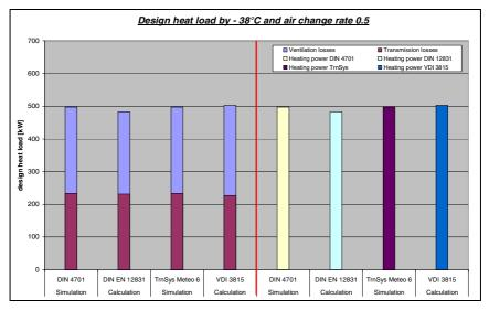
Fig. 9. Identified maximum heat load at -38  $^{\circ}$  C
