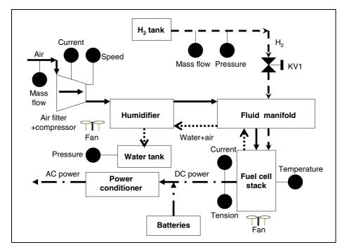
Fig. 1. Scheme of fuel cell stack system
