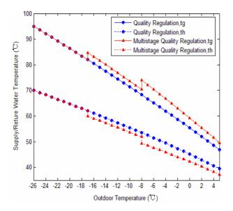
Fig. 1. Regulated curve of teaching building during normal use
