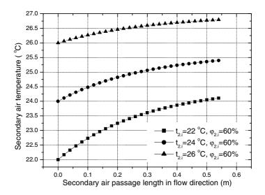
Fig. 5. Temperature distribution of secondary air
