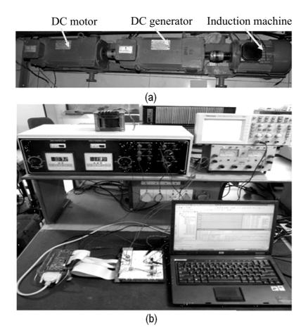
Fig. 4. (a) DC motor-generator set; (b) Control circuitry and DC motor drive
