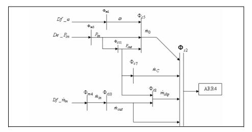
Fig. 6. Oriented graph for hydraulic part of the compressor
