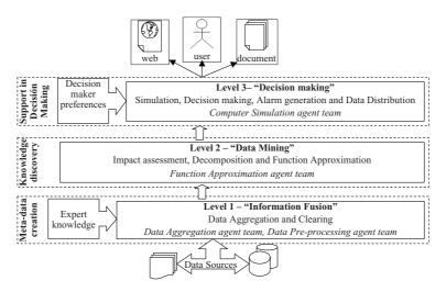
Fig. 4. The general architecture of the decision making system
