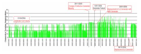
Fig. 3. Daily maximal temperature of generator bearing
