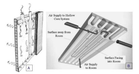
Fig. 6. A Murocaust apartment Block in Gothenburg (Hastings and Mørk 1999) B Hypocaust Thermo deck system (Barton et al. 2002)
