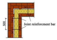
Fig. 8. Connecting structure of the wall
