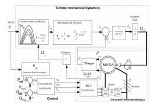
Fig. 6. Block diagram of the studied system
