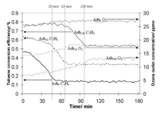
**Fig. 2.** Toluene conversion efficiencies and outlet ozone concentrations over various FAP. Experimental conditions: Toluene, 1.5 ppmv; Ozone, 36 ppmv; Mass of FAP, 1 g; Residence time, 0.15 s; Temperature, 24-26 °C.
