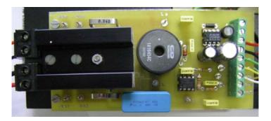
Fig. 10. Power block of PV system
