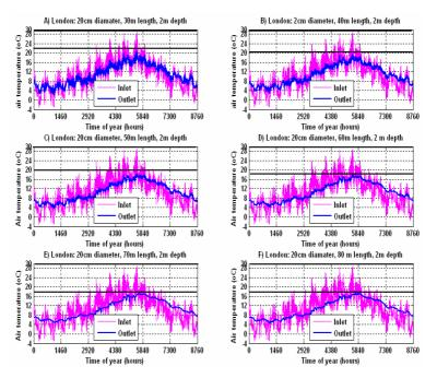
Fig. 4. Air temperature for London; EAHX 30m to 80m long, 2 m/s air velocity
