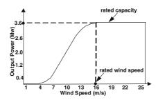
Fig. 3. A typical machine power curve
