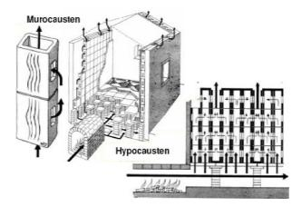
Fig. 1. The Roman thermo- and muro-causten system (Florides et al. 2002)
