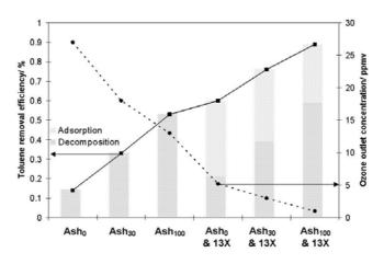
**Fig. 4.** Effect of the combined use of FAP and zeolite 13X on steady state toluene conversion efficiency and ozone outlet concentration. Experimental conditions: Toluene, 1.5 ppmv; Ozone, 36 ppmv; Mass of FAP, 1 g; Mass of Zeolite, 1 g; Residence time, 0.15 s (FAP only), 0.22 s (FAP+13X); Temperature, 24-26 °C.
