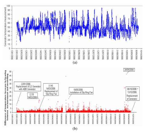
Fig. 5. Bearing temperature obtained from neural networks modelling method
