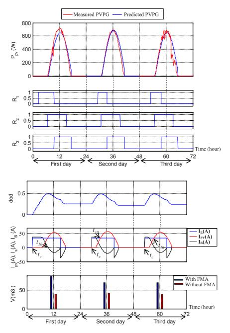
**Fig. 5.** The experimental results for the typical day: a) The PVP Generation and the relays switching, b) The battery *dod*, the current assessment, the pumped water
