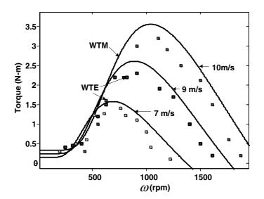
Fig. 10. Experimental Results: Comparison of Torque-Speed characteristics obtained using WTM and WTE
