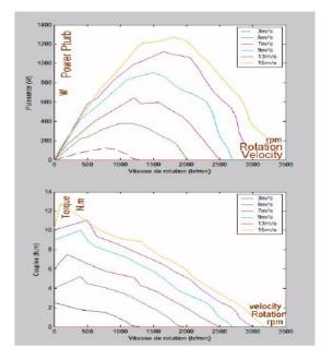
Fig. 7. Simulation results : Power and Torques Vs velocity rotation
