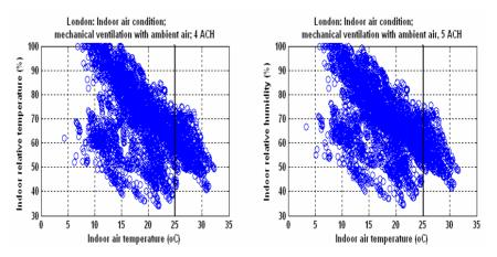
Fig. 5. Indoor air condition for ventilation with ambient air
