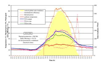
Fig. 9. Experimental results (stabilized electrical source) for the French-window shutter
