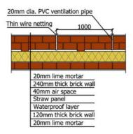
Fig. 5. Detail drawing of wall ventilation
