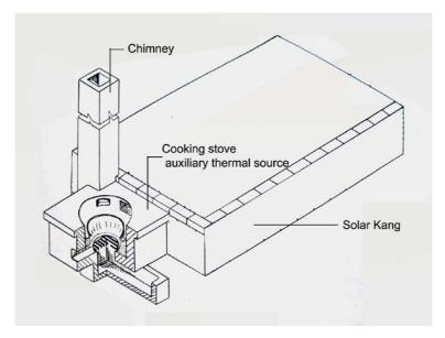
Fig. 4. Auxiliary thermal source
