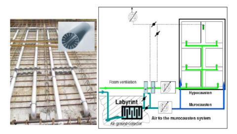
**Fig. 7.** The concrete core activating system ConcreteCool and Principe schematic of the hypocausten /murocausten system in combination with air-ground collector and labyrinth foundation collector
