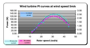
Fig. 5. Wind turbine power current curves at wind speed 5m/s
