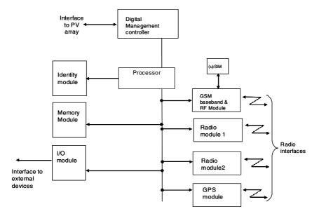
Fig. 2. Block diagram of control module
