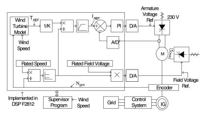
Fig. 2. Control diagram of the torque control scheme
