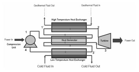
Fig. 2. Geothermal power cycle flow diagram [13]
