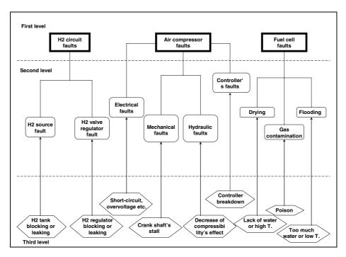
Fig. 2. Faults tree of fuel cell stack system
