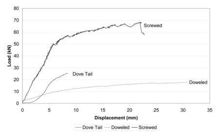
Fig. 3. Joint Testing Results
