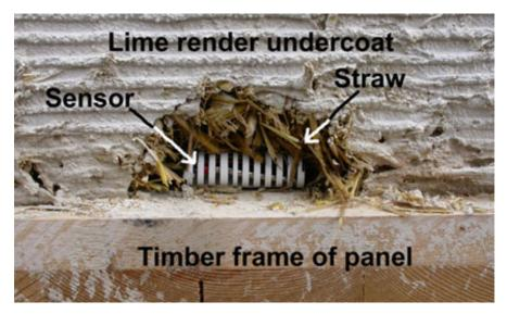
Fig. 3. Sensor inserted just below the external render (prior to final rendering)
