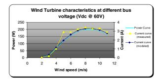
Fig. 4. Comparison of modeled wind turbine characteristics against measured data ( $V_{DC} = 60V$ )
