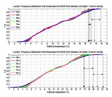
Fig. 3. London: Frequency distribution of Outlet air temperature, 30-80m length
