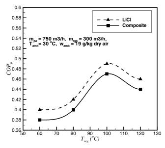
Fig. 3. Regeneration temperature vs. system performance
