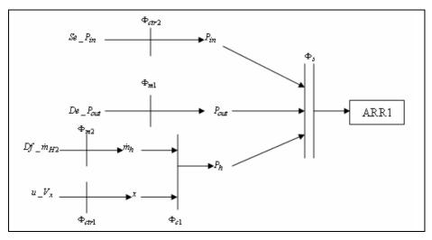
Fig. 3. Oriented graph for H<sub>2</sub> valve
