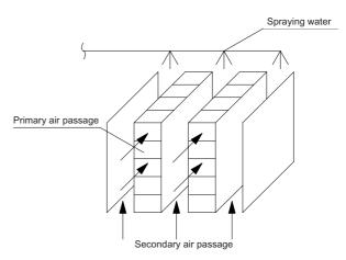
Fig. 1. Structure of the cross-flow plate heat exchanger for evaporative cooling
