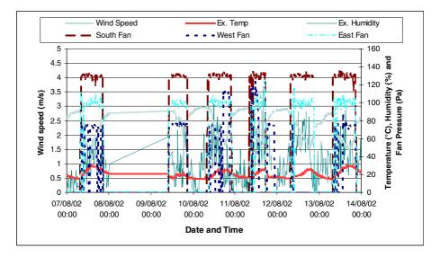
Fig. 4. Plotted external wind speed against fan pressure and external temperature and humidity
