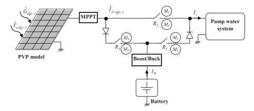
Fig. 3. The switching strategy for the PVP/ Battery/Load system
