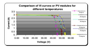
Fig. 3. Comparison of emulated and theoretical PV module curves ( $I_{sc} = 3A$ )
