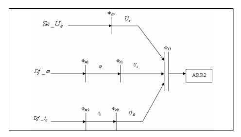
Fig. 4. Oriented graph for electric part of the compressor
