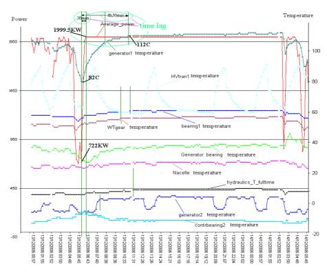
Fig. 2. The lag between temperature and power
