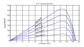
Fig. 3. P-V characteristics with insulation variations and constant cell temperature
