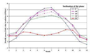
Fig. 11. Monthly mean values of the daily solar irradiation on tilted planes for Ajaccio calculated by Calsol Software (INES 2008)
