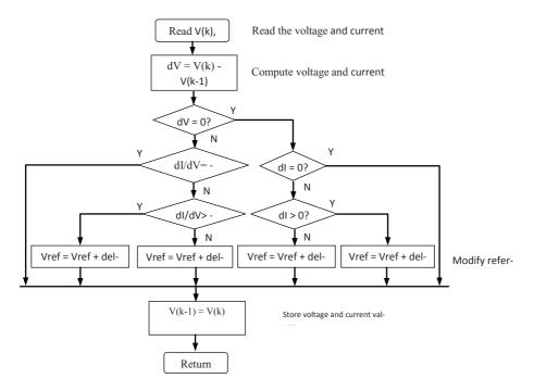
Fig. 8. Flow chart of the MPPT Incremental Conductance Method
