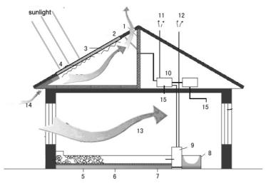
1. Adiabatic and shading board; 2. Opened damper; 3. Heat-gathering glass; 4. Automatic sunshade device; 5. Flue; 6. Heat-insulated layer of flue; 7. Remaining heat of cooking; 8. Cooking stove; 9.furnace; 10. Heat-recycling devices; 11. Dirty air; 12. Exit of burning production; 13. Draught; 14. Fresh air comes into the heat collection device through the eaves; 15. Exit of dirty air
