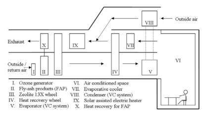
Fig. 5. Schematic diagram of the air purification and desiccant cooling system
