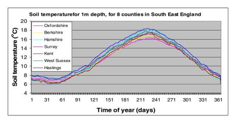
Fig. 1. Annual soil temperature profile for South East, UK
