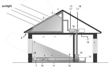
1. Adiabatic and shading board; 2. Closed damper; 3. Heat-gathering glass; 4. Fresh air comes into the heat collection device through the eaves; 5. Hot air screen; 6. Exit for hot air; 7. Gravel storage heat; 8. Thermolysis; 9. Heat from heat-collection device; 10. Flue 11. Heat-insulated layer of flue; 12. Remaining heat of cooking; 13. Cooking stove; 14. Furnace; 15. Smoke and humidity of cooking; 16. Heat-recycling devices; 17. Dirty air; 18. Exit of burning production;
