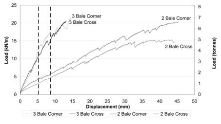
Fig. 5. ModCell Panel Racking Shear Testing Results
