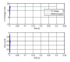
Fig. 13. The response of output voltage and the control input
