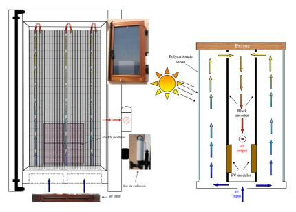
Fig. 5. The solar collector, its main components and the air circulation
