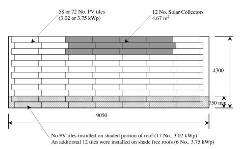
Fig. 2. Roof plan showing PV layout
