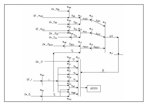
Fig. 8. Oriented graph for electric part of fuel cell
