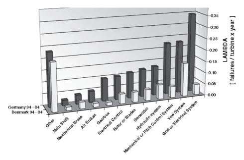
Fig. 1. Average failure rate of wind turbine components
