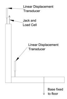
Fig. 2. Joint Testing Set up
