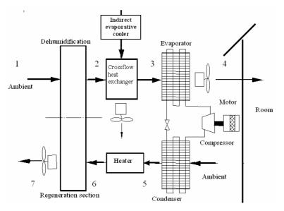
Fig. 1. Schematic of the hybrid system
