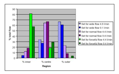
Fig. 3. The effect of flow-rate change in an adjustable shower head
