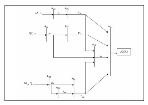
Fig. 5. Oriented graph for mechanic part of the compressor
