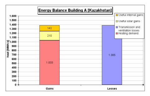
Fig. 11. Energy balance of the building with weather data of Ust- Kamenogorsk, Kazakhstan
