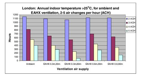
Fig. 7. Indoor temperature exceeding 25°C, EAHX and ambient air ventilation
