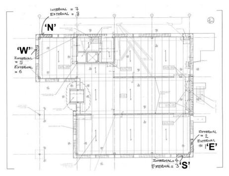
Fig. 4. Location plan of sensors on the building
