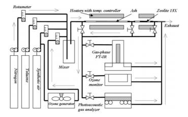
Fig. 1. Schematic diagram of the fixed bed flow reactor
