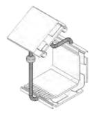
Fig. 5. Type 4:collector to murocaust and hypocaust (Hastings 1998)
