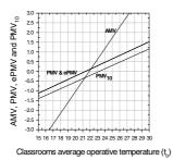
**Fig. 4.** The regressed neutral temperature  $(t_n \text{ of the girls' AMV} and the different predicted indices (PMV, ePMV and PMV_{10})$
