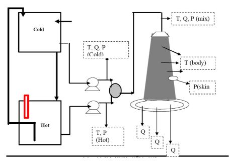
Fig. 1. Schematic view of laboratory trial system
