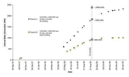
Fig. 4. PV performance over 12 month period for two properties
