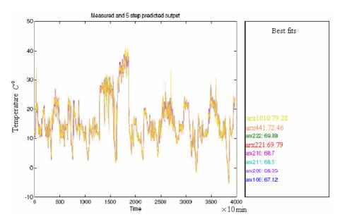
Fig. 4. Black-box modelling of bearing temperature
