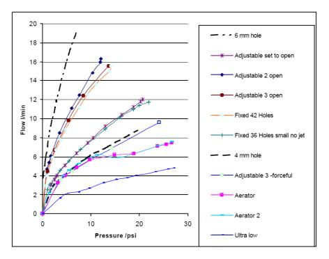
Fig. 2. Pressure-flow relationships. In some cases very high flow rates (over 12 l/min) were achieved at moderate or high pressures, whereas aerated showerheads and low flow showerheads maintained flows below 8 l/min even at the highest pressures.
