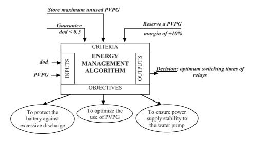
Fig. 1. The synoptic schema of the proposed approach
