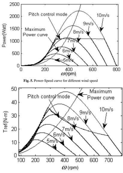
Fig. 6. Torque-Speed curve for different wind speed
