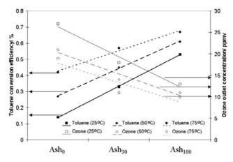
**Fig. 3.** Effect of temperature on steady state toluene conversion efficiency and ozone outlet concentration over various FAP. Experimental conditions: Toluene, 1.5 ppmv; Ozone, 36 ppmv; Mass of FAP, 1 g; Residence time, 0.15 s; Temperature, 25-75 °C.
