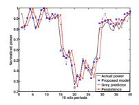
Fig. 6. Normalized wind power predictions for different models
