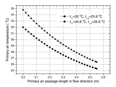
Fig. 4. Temperature distribution of primary air
