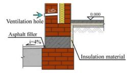
Fig. 7. The connection fabric between exterior wall and floor
