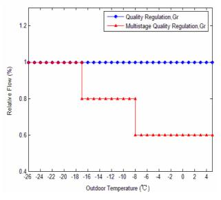
Fig. 2. Relative flow of teaching building during normal use
